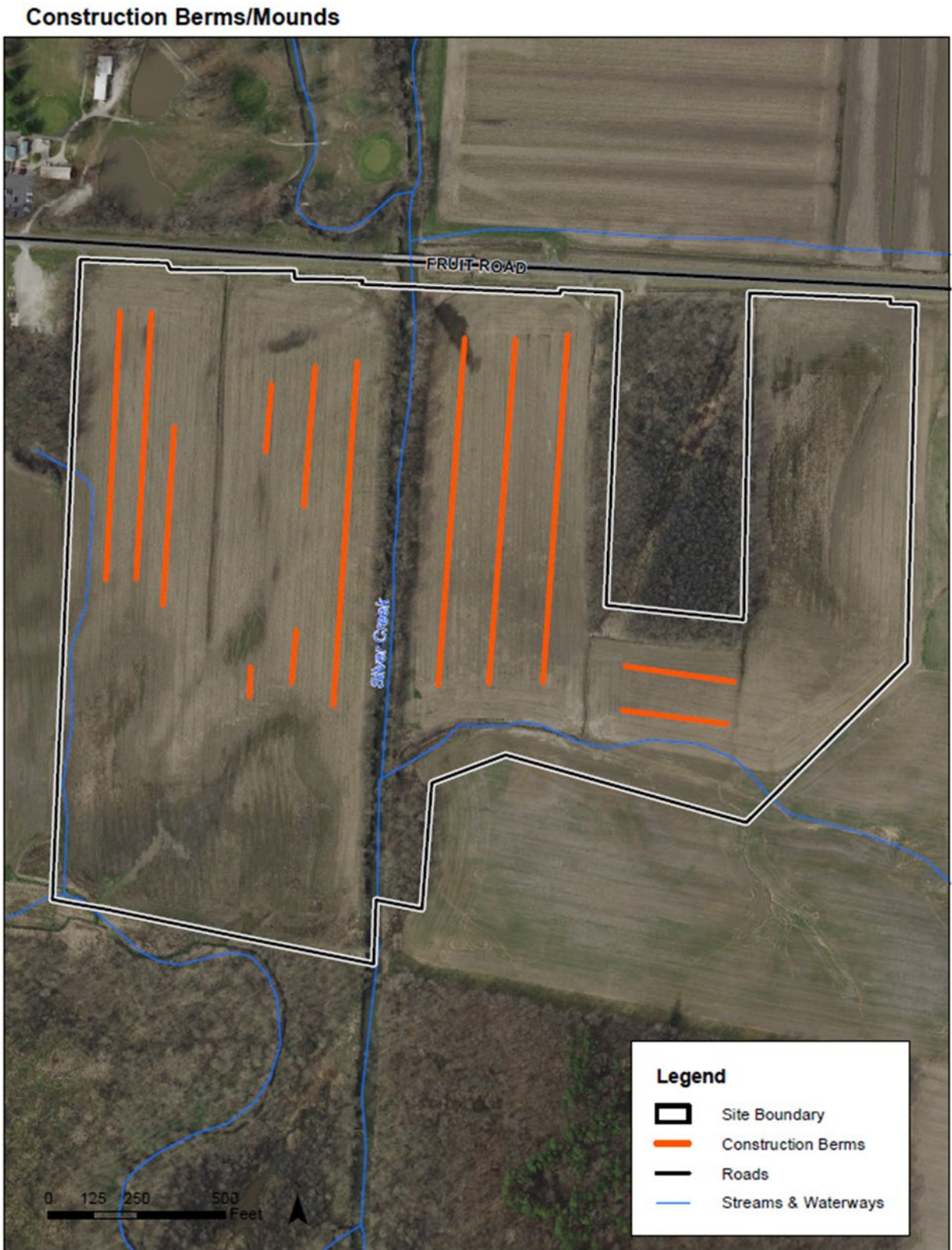
Figure 13 – Berm Construction Features for Tree Planting
