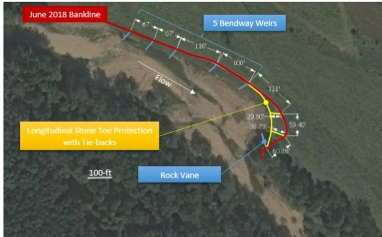
1. 5 Bendway Weirs (480-tons) to control conveyance of flow energy
