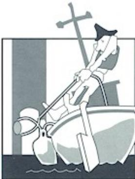
7. Secure both lines around the mooring bitt so they may be released quickly, *in case the bitt gets stuck.* Keep careful watch throughout the lockage. *In case of emergency, you could be told to quickly release your vessel from the mooring bitt.* Please remain secured to bitt until told to proceed.
