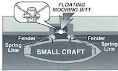
1. Receive permission to enter the lock either verbally from the lock operator or from horn and signal lights. Proceed into the lock and tie up at the mooring bitt designated by the lock operator. *Make sure you secure your vessel to the **FLOATING MOORING BITT** and not to a ladder or other immovable device.*
