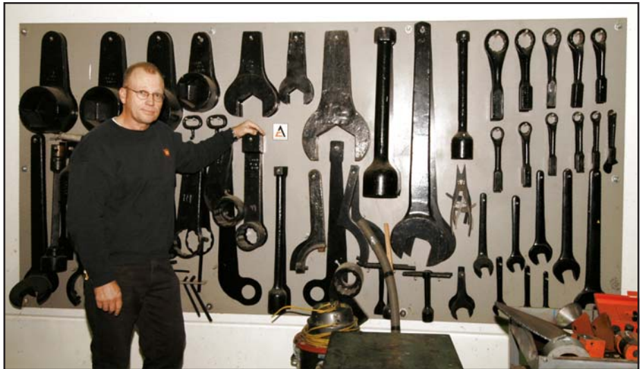
Mechanic Kevin Long shows some of the massive sockets and wrenches necessary to maintain and repair the giant machinery of Cannon Power Plant.
