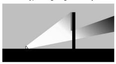
The preferred method for lighting a sign panel is using concealed ground-mounted fixtures. This provides enough light without glare or over glow.
