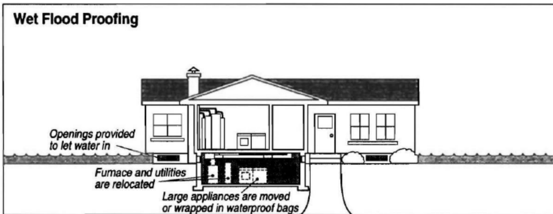
Figure 2. Nonstructural Wet Floodproofing Diagram
