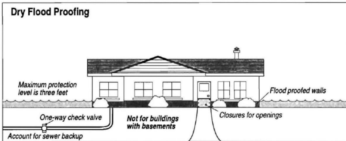
Figure 1. Nonstructural Dry Floodproofing Diagram
