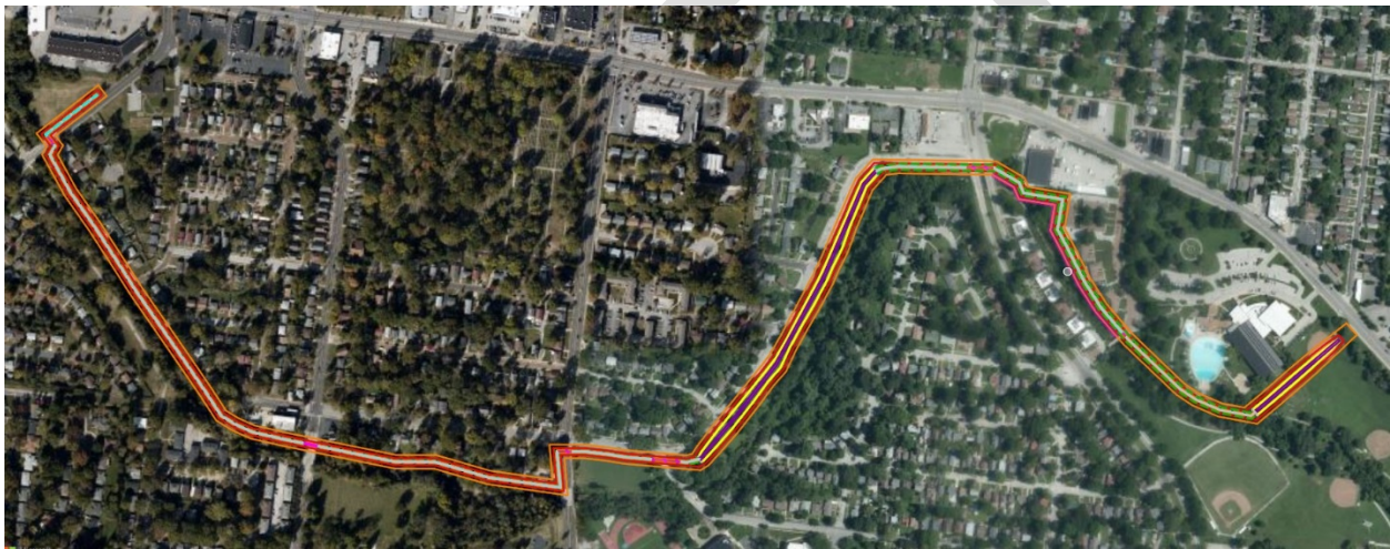
Figure 6. Plan View of the Combination Earthen Levee – Concrete Floodwall Alignment
