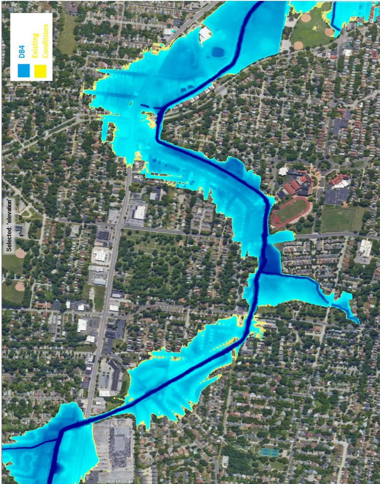
Figure 21. Proposed DB4 Alternative versus Existing Conditions Inundation - 1% AEP - Groby/Shafsbury/Wilson Vicinity
