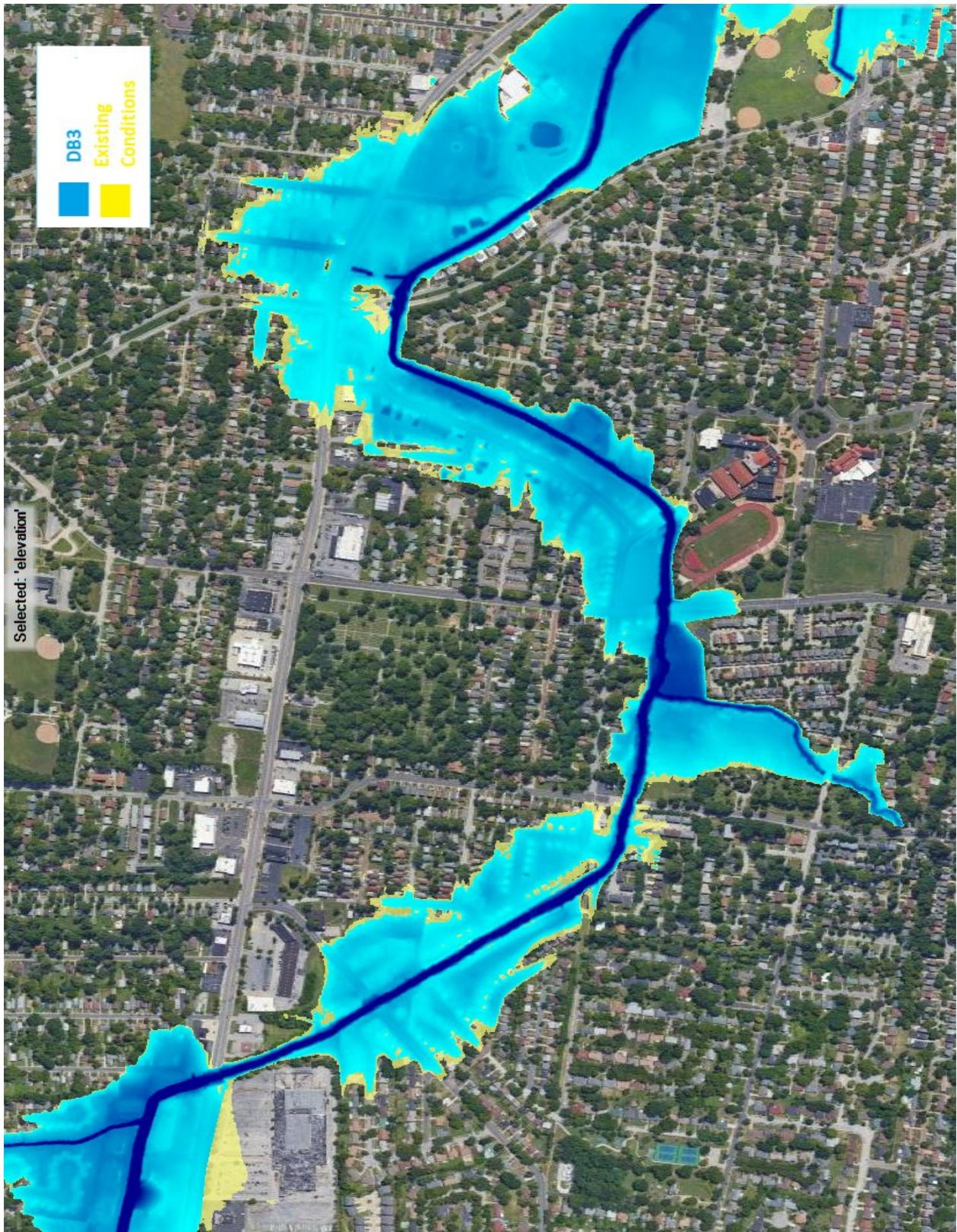
Figure 20. Proposed DB3 Alternative versus Existing Conditions Inundation - 1% AEP - Groby/Shafsbury/Wilson Vicinity
