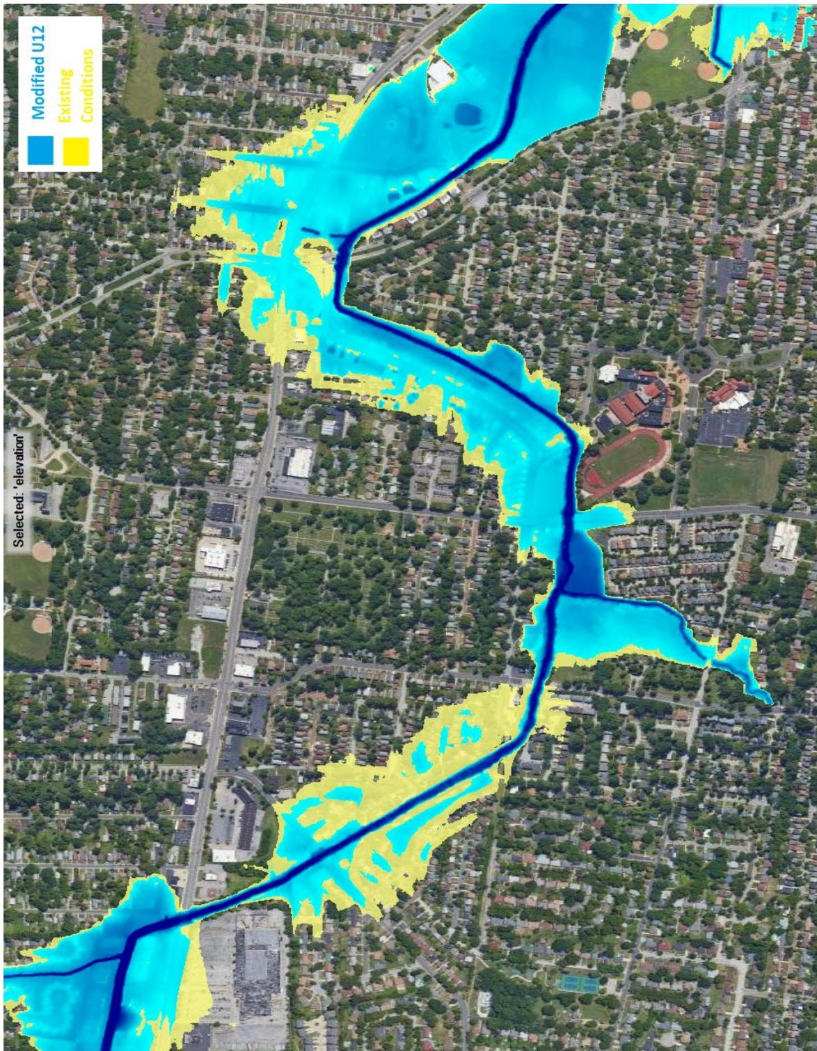
Figure 25. Proposed Modification to U12 Alternative versus Existing Conditions Inundation - 1% AEP - Groby/Shafsbury/Wilson Vicinity
