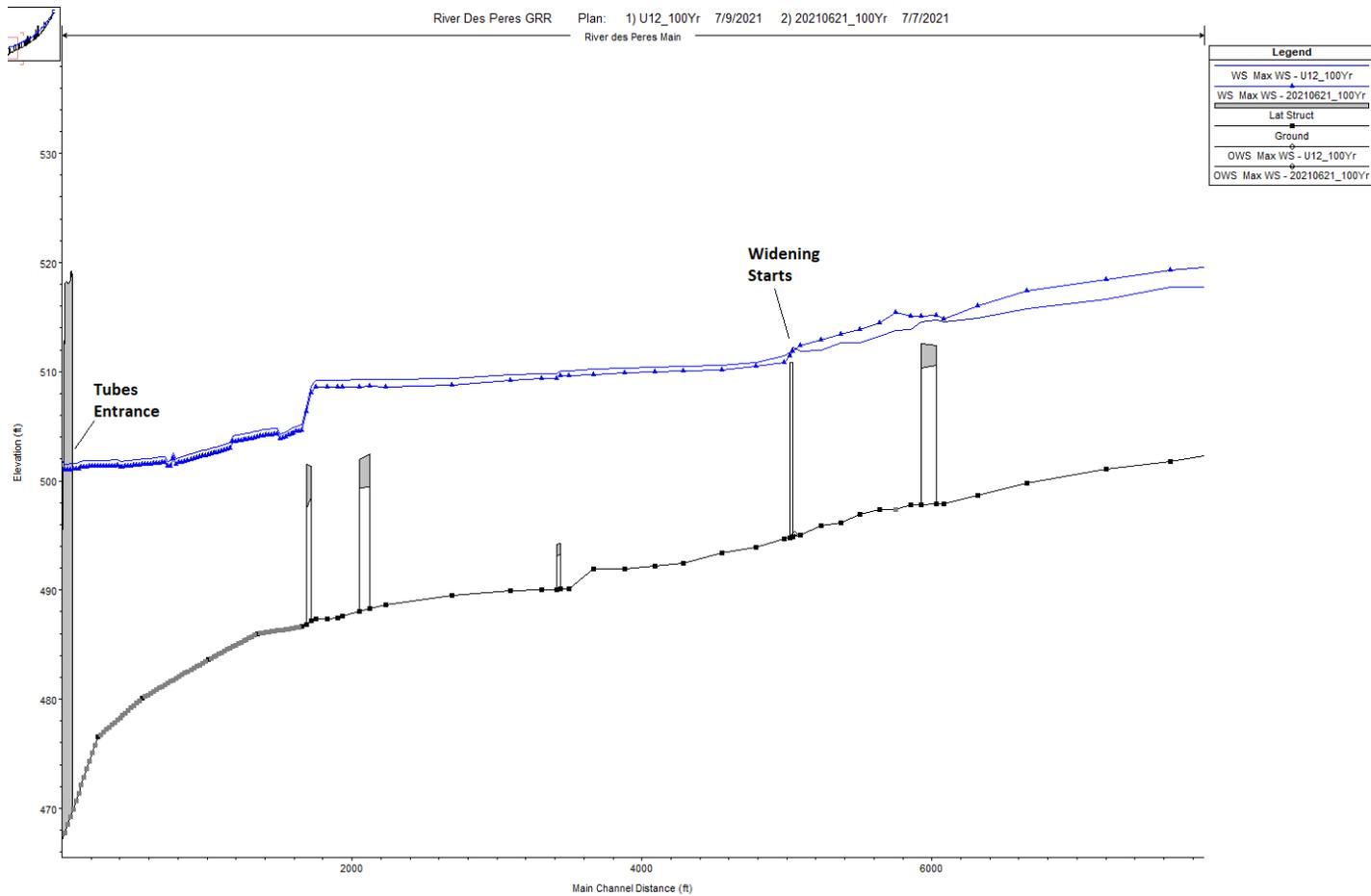
Figure 23. Original TSP, Alternative U12, Channel Widening - 1% AEP Water Surface Profile
