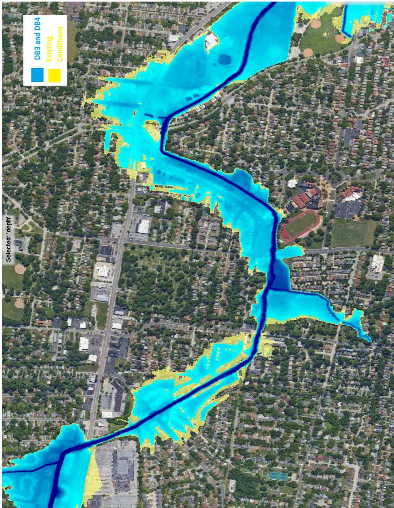
Figure 19. Proposed DB3 and 4 Alternative versus Existing Conditions Inundation - 1% AEP - Groby/Shafsbury/Wilson Vicinity
