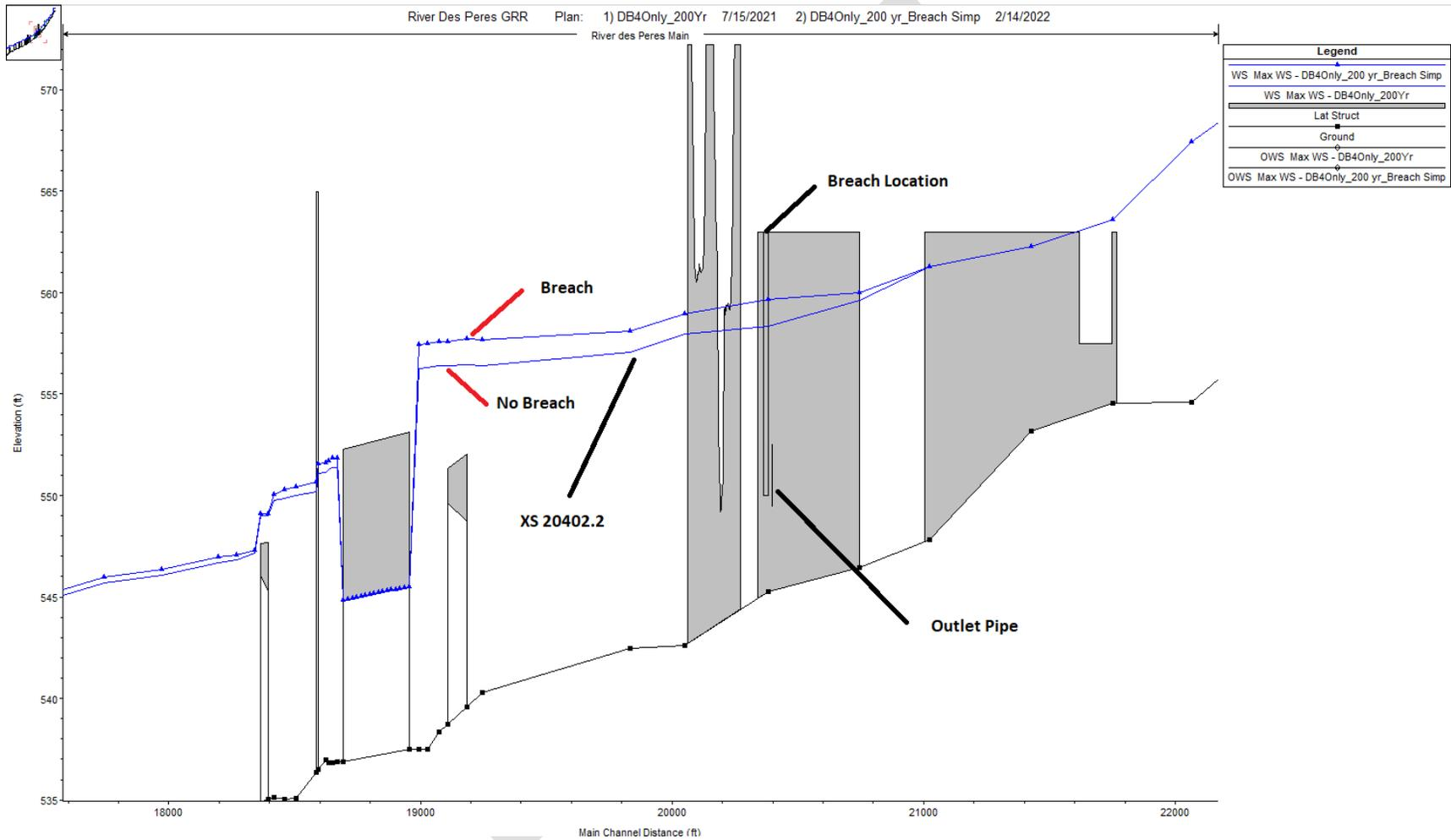
Figure 26 – 0.5% AEP With-Project Breach versus No-Breach
