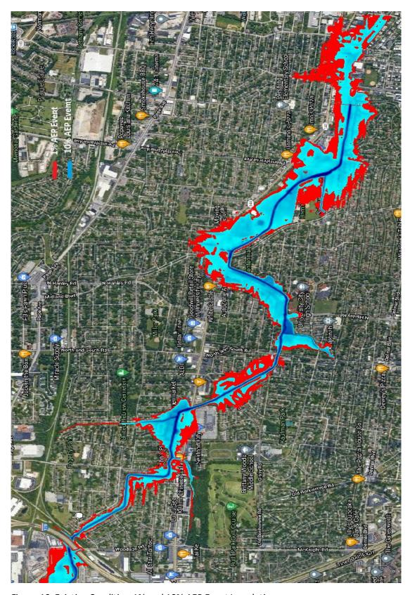
Figure 10. Existing Condition 1% and 10% AEP Event Inundation
