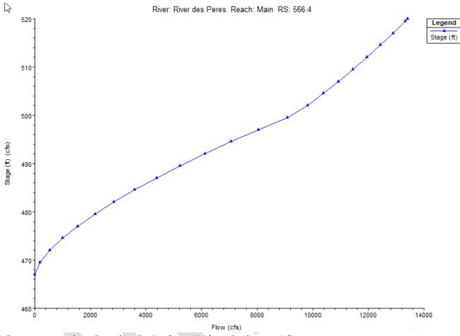
Figure 5. Downstream culvert Boundary Rating Curve Without Backwater Adjustment
