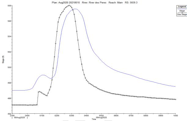
Figure 7. Computed versus observed water surface at River Des Peres, University City gage August 2020
