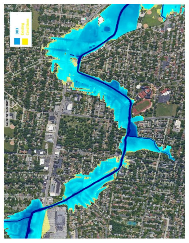
Figure 20. Proposed DB3 Alternative versus Existing Conditions Inundation - 1% AEP - Groby/Shaftsbury/Wilson Vicinity
