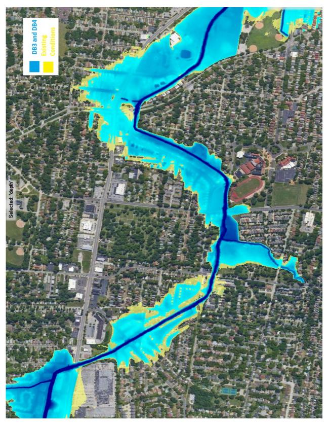
Figure 19. Proposed DB3 and 4 Alternative versus Existing Conditions Inundation - 1% AEP - Groby/Shaftsbury/Wilson Vicinity
