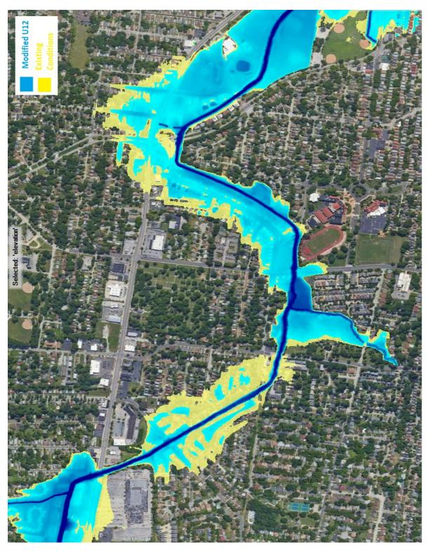
Figure 25. Proposed Modification to U12 Alternative versus Existing Conditions Inundation - 1% AEP - Groby/Shaftsbury/Wilson Vicinity
