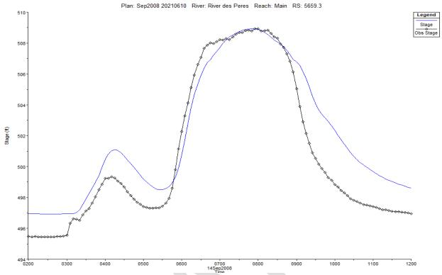
Figure 8. Computed versus observed water surface at River Des Peres, University City gage September 2008
