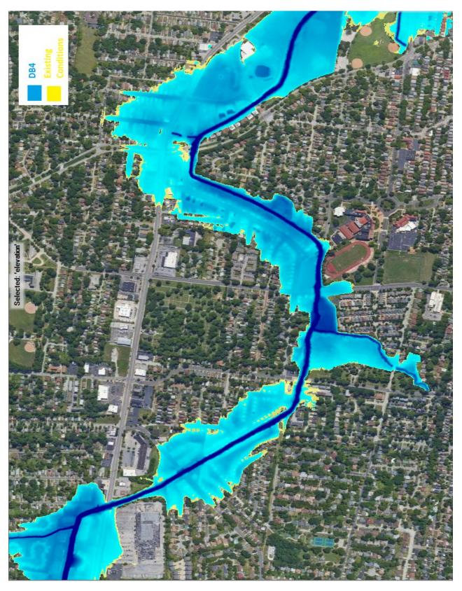
Figure 21. Proposed DB4 Alternative versus Existing Conditions Inundation - 1% AEP - Groby/Shaftsbury/Wilson Vicinity
