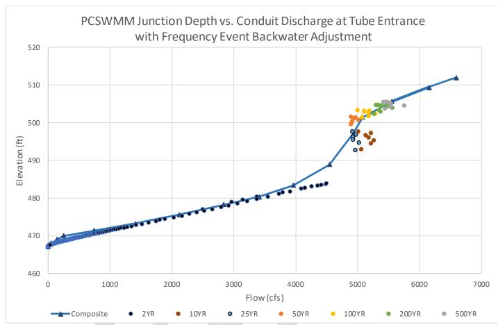
Figure 6 - Adjusted Rating Curve at Tube Entrance Accounting for Backwater Influence
