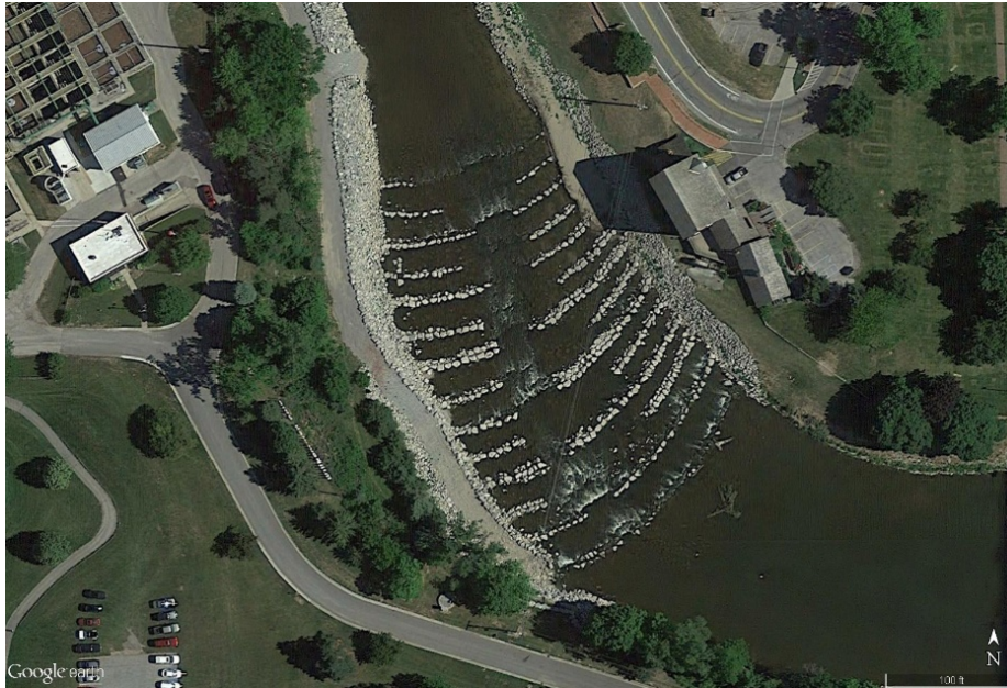
Figure 2-19: Frankenmuth, MI, Engineered Rock Riffle with Integrated Weirs, Google Earth 2016
