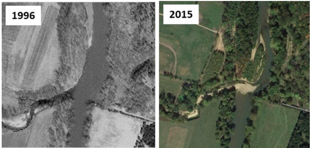
Figure 2-1. Channel Instability Into Right Descending Bank Due to Delta Formed Confluence of Ditch Creek and Big River at RM 44.5 (Flow From Bottom to Top)
