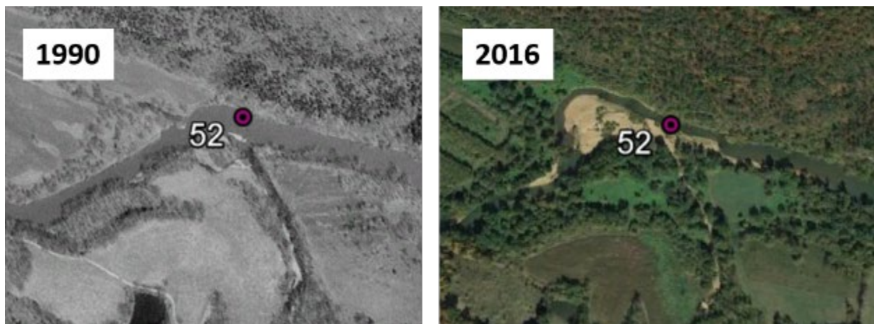
Figure 2-3. Channel Instability Into Right Descending Bank Due to Delta Formed Confluence of Calico Creek and Big River at RM 52 (Flow From Right to Left)
