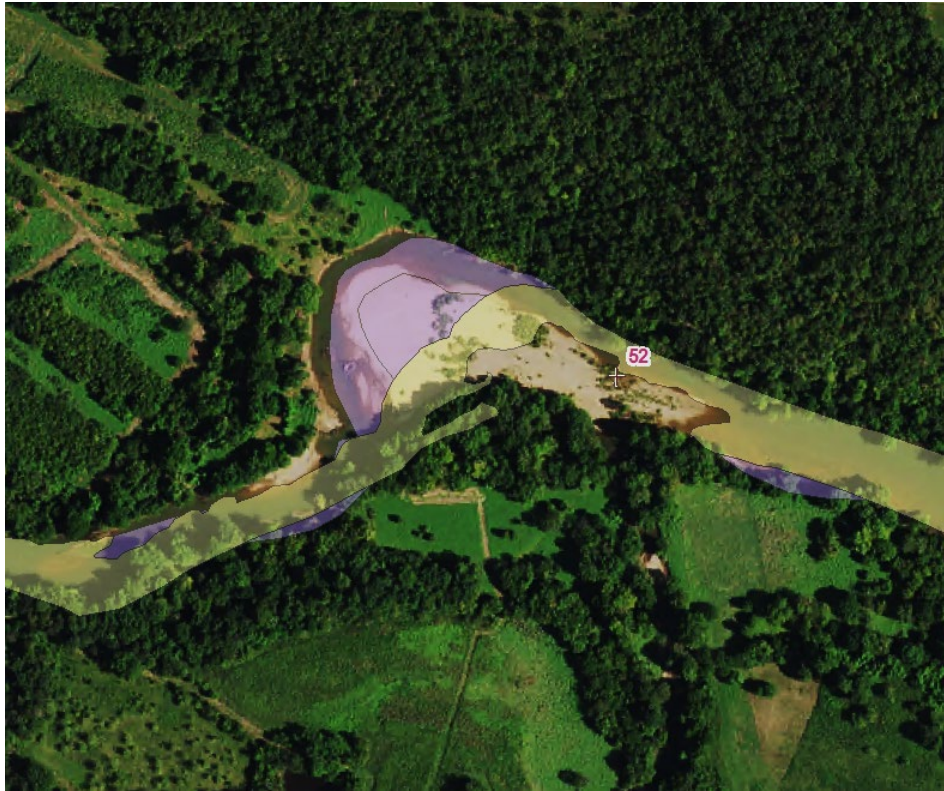
Figure 3-7. Step 1: Identify Eroded Area. Yellow is old channel; purple is new channel + area through which the old channel eroded
