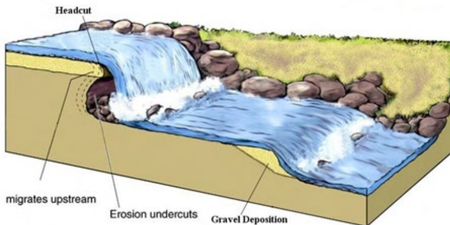
Figure 2-18: Diagram of a Head-Cut (NYDEC, 2014)
