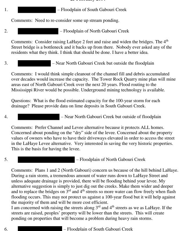
Comments: I favor the authorized plan with the 20' ditch with 2:1 slopes but I feel that the only way to get full benefit from this is to change the RR bridge at Main Street to a wider span for the supports at the channel to get them out of the channel. The skew of the supports may need to be change too. If all this isn't done the debris against the existing supports will continue to act as a dam.
