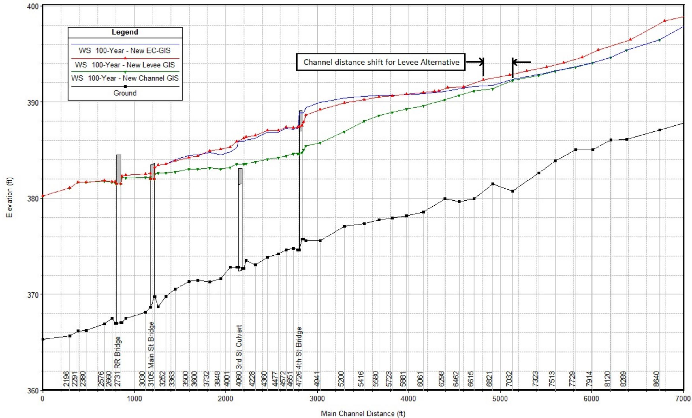
Notes: 1. The profile plot for the Levee plan is shifted to the left of the Existing Conditions profile, because it also includes a channel realignment that shortens the main channel distance by about 300 feet.
