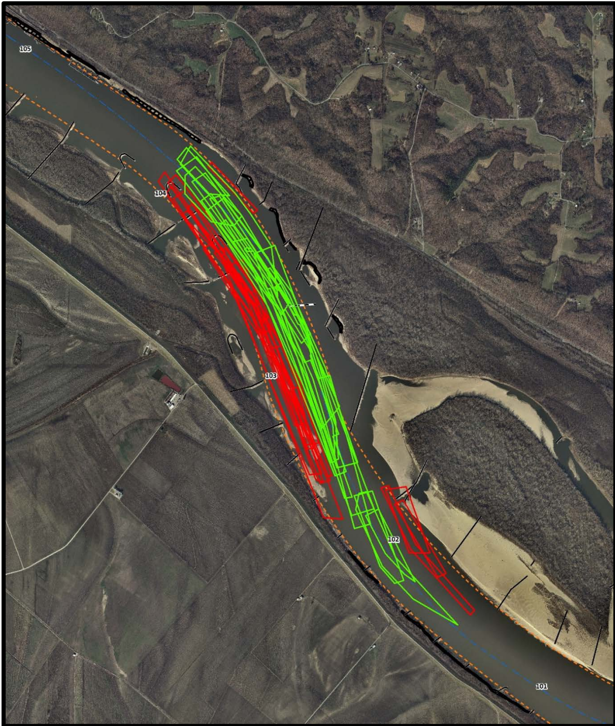
Figure 2. Approximate location of the 17 channel maintenance dredging events (green) and dredge disposal locations (red) performed in the work area from 2000 to 2015.
