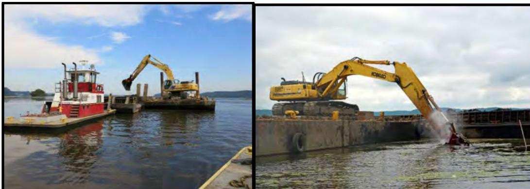
**Figure 5-2. Example of barge mounted excavator**
