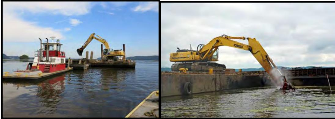
**Figure 5-2. Example of barge mounted excavator**
