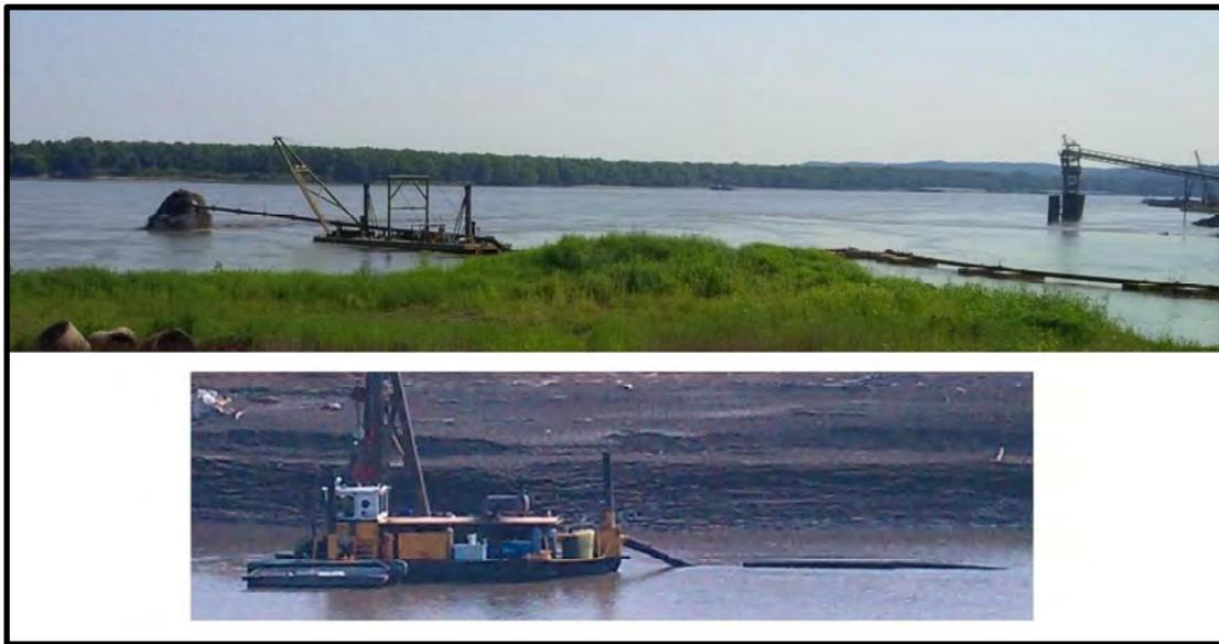
Figure 5-1. Example of hydraulic cutterhead dredge and pontoon pipeline
