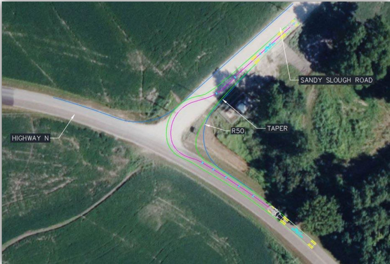
Figure 10. Required road improvements at the intersection of Highway N and Sandy Slough Road.
