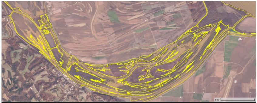
Figure 20. Inundation Boundary Comparison for WSE at Chester of ~365 ft NAVD88 on February 25, 2018
