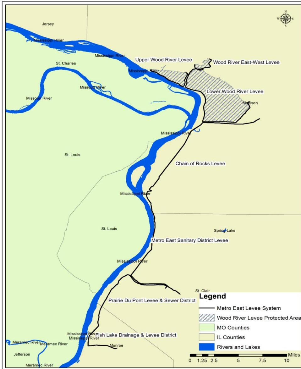
Figure 1: Metro East Levee system in Illinois which consists of Wood River Levee system, Chain of Rocks, Metro East Sanitary District, Prairie Du Pont Levee, and Fish Lake Drainage and Levee District. The Wood River Levee system consists of Upper, Lower, and East-West levees.
