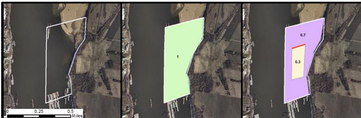
Figure 5. Delineation of the total area of influence (left) as well as pre- (center) and post-construction (right) delineation of the structured/unstructured parameter categories for the Mosenthein Ivory Landing Phase 4 work area. Construction of the rootless dike (red) reduces the score immediately downstream of the dike to 0.3, and the remainder of the area to 0.7, because a dike is now present within the total area of influence.
