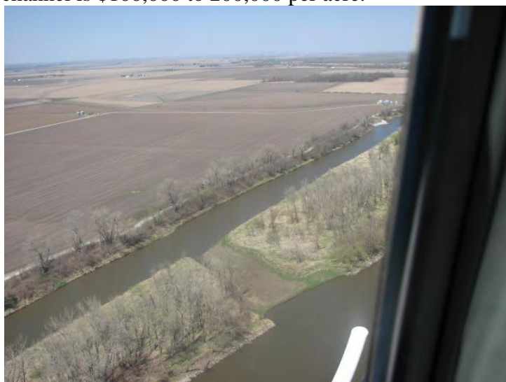
Figure P: River tie-back channel during low water
