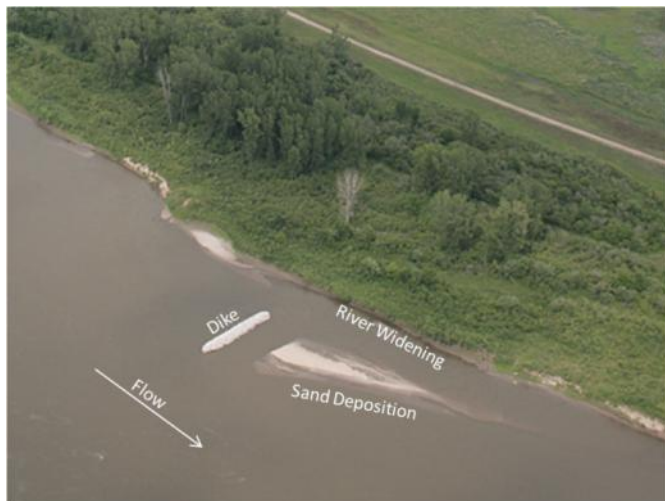
Figure J: Aerial view of a rootless dike.
