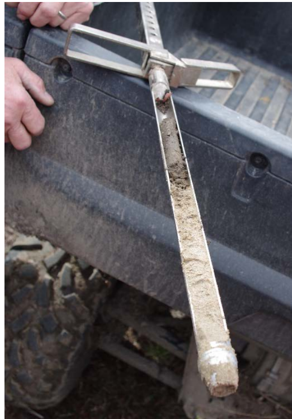
Figure 7: Soil Probe Sample from Behind Wilkinson Island Breached Levee
