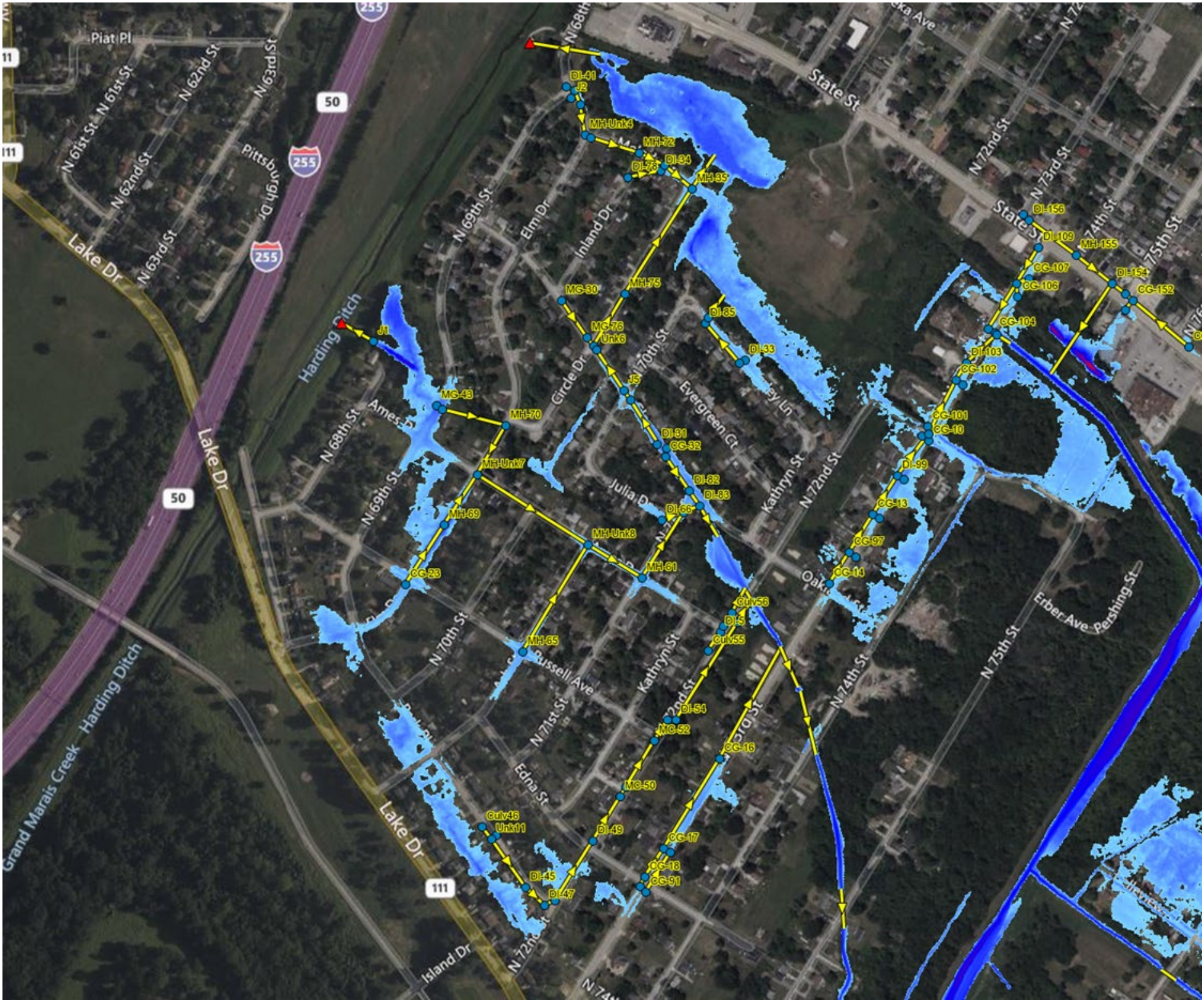
Figure A- 18: Parkside Watershed Existing Conditions Inundation - 10% AEP
