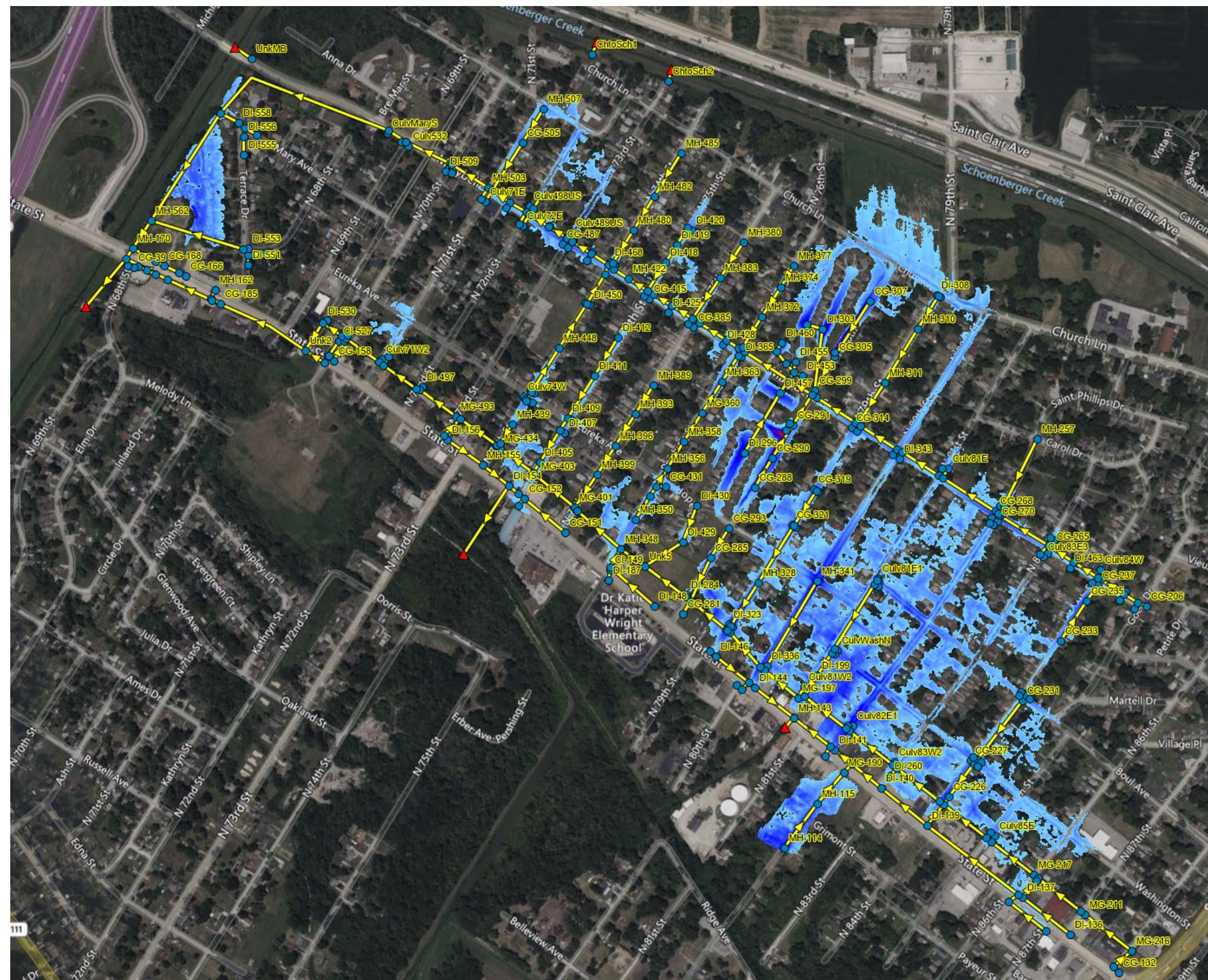
Figure 31: Edgemont Watershed- Existing Conditions- 10% AEP
