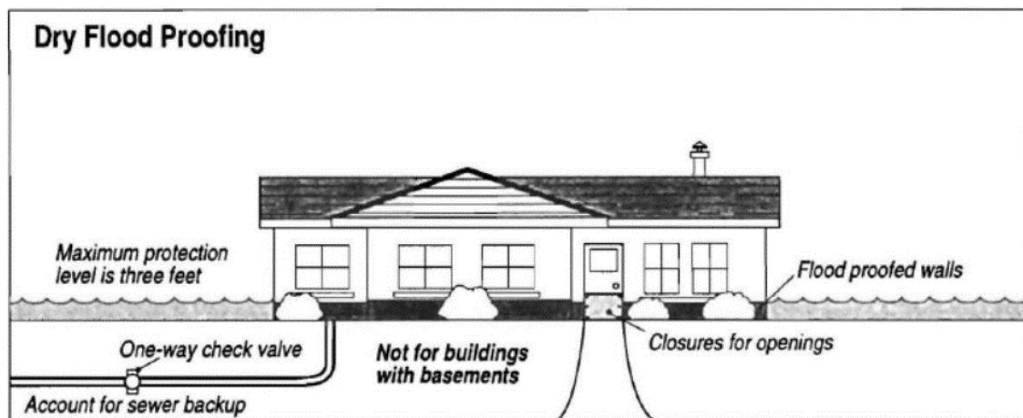
Figure 27: Dry Flood Proofing Diagram
