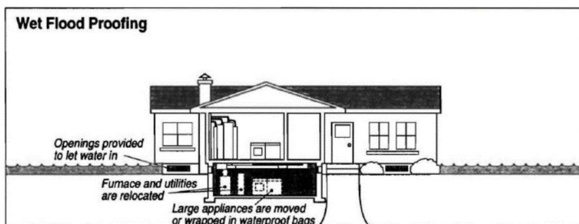
Figure 28: Wet Flood Proofing Diagram
