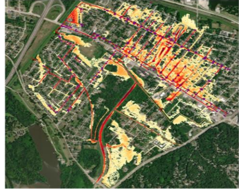
Figure 1: Surface flooding from a 1% Annual Exceedance Probability storm producing 7.65 inches of rain in 24-hour period
