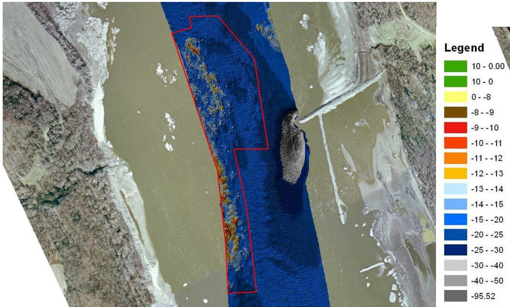
Figure 14: Work Area TR9P is located at approximately River Mile 41.0. This work area consists of limestone pinnacle rock. All material above an elevation of 289.1 ft NGVD 1929 (-13 ft design plane) is to be removed. The estimated quantity of material to be removed is 115 cubic yards.
