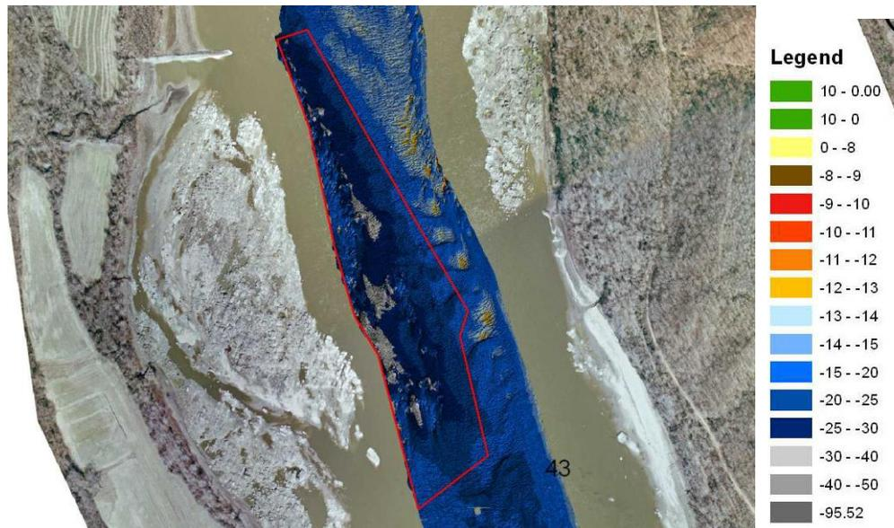
Figure 13: Work Area TR8P is located at approximately River Mile 42.8. This work area consists of both limestone shelf rock and pinnacle rock. All material above an elevation of 290.1 ft NGVD 1929 (-13 ft design plane) is to be removed. The estimated quantity of material to be removed is 187 cubic yards.
