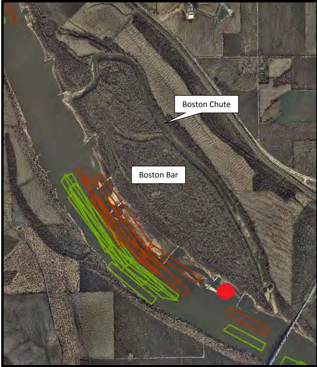
Figure 3. Approximate location of channel maintenance dredge cuts (green boxes) and dredge disposal locations (red boxes) performed in the Boston Bar vicinity since the year 2000, and the proposed location for future dredge disposal (red circle).
