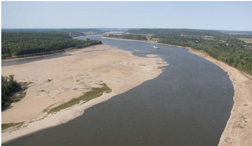
Figure 2. Drought and low water on the Middle Mississippi River meant exposed sandbars, hazards for navigation, and a narrow navigation channel.
