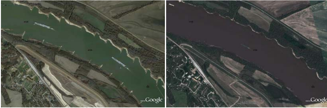
Figure 2: (left) river training structures at low flow (right) river training structures at above average flow (approx)
