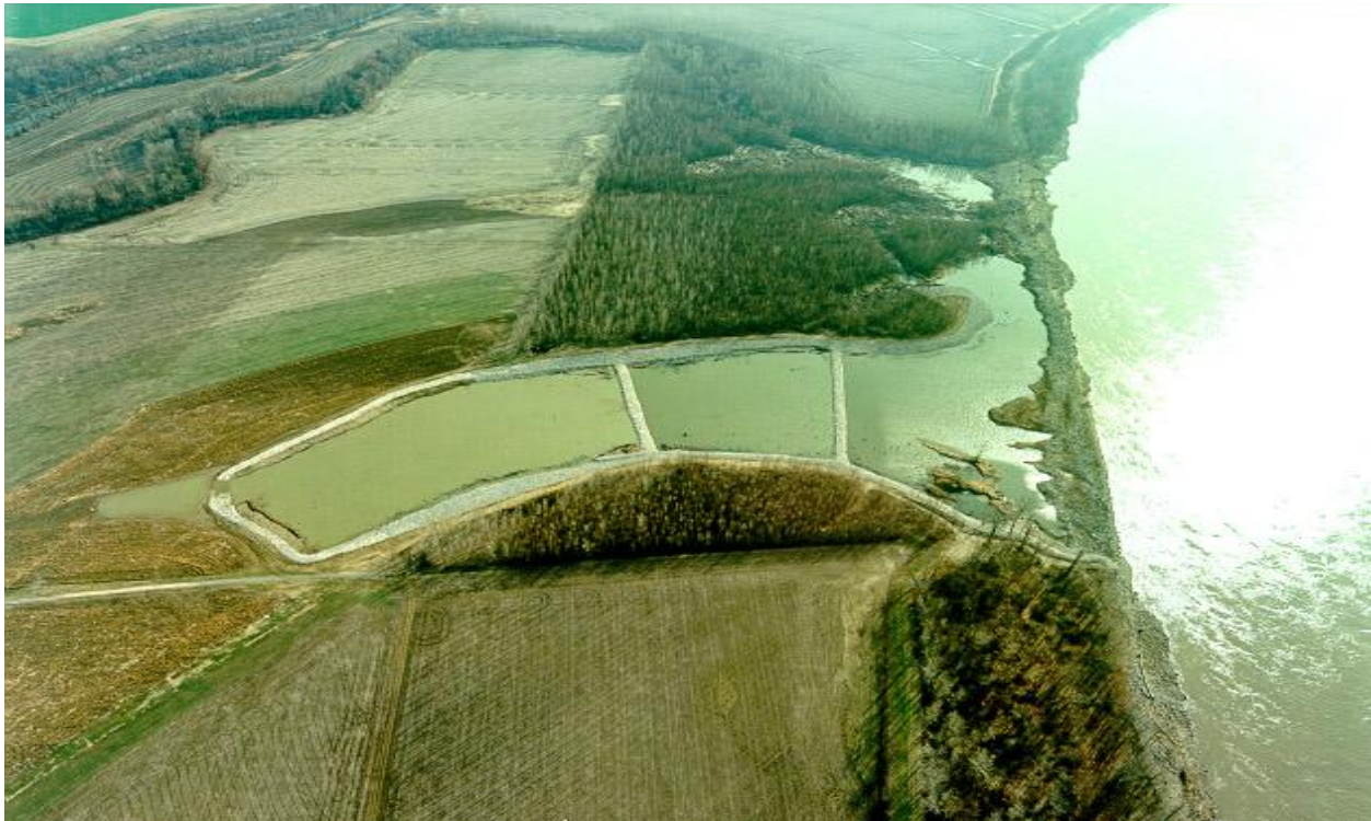
Figure 26: Tree Screens and Baffles at Upper and Lower Dry Bayou Scour Holes in 2000
