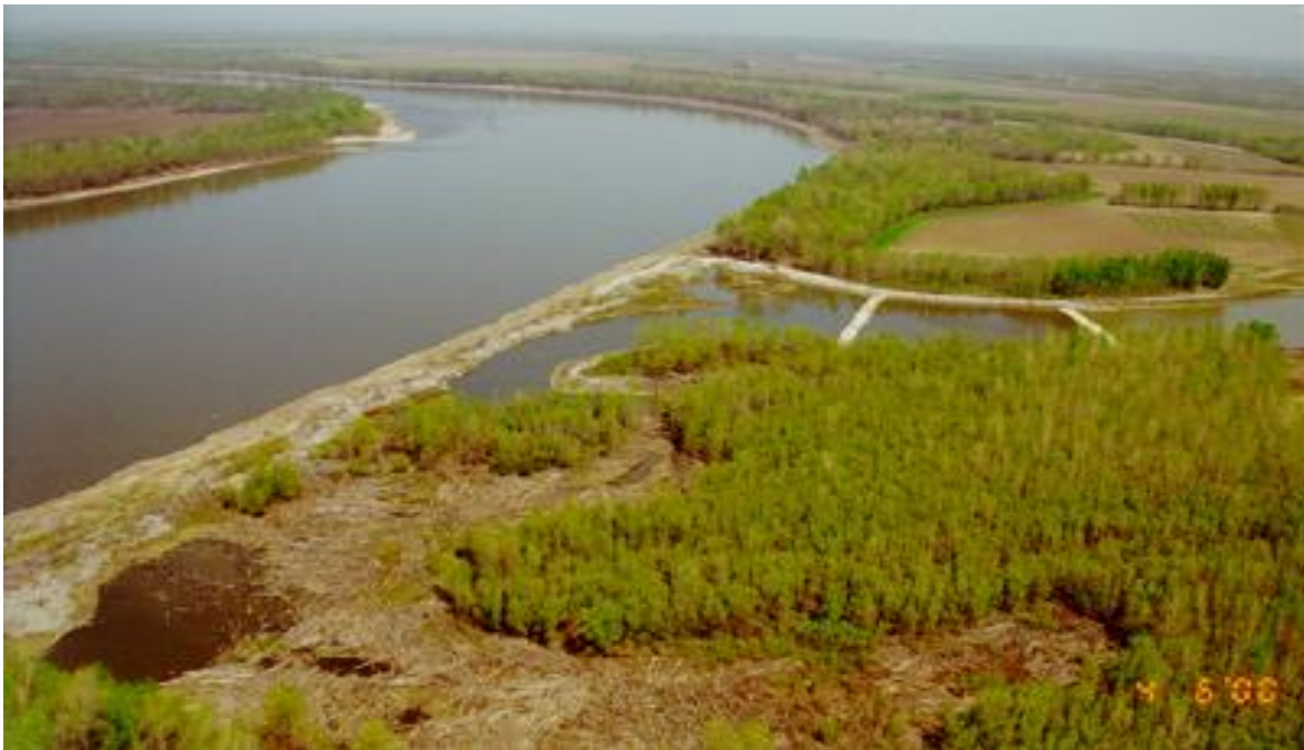
Figure 28: Tree Screens and Baffles at Upper and Lower Dry Bayou Scour Holes in 2000
