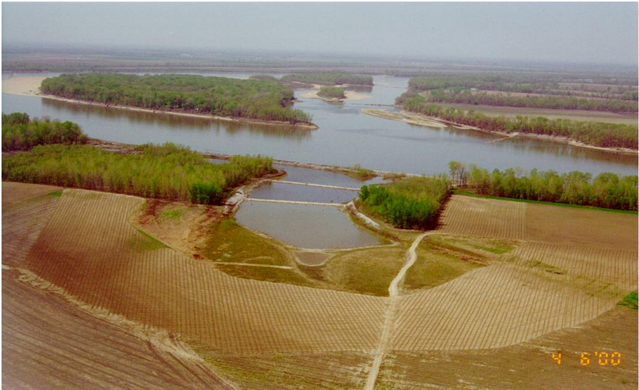
Figure 27: Tree Screens and Baffles at Upper and Lower Dry Bayou Scour Holes in 2000
