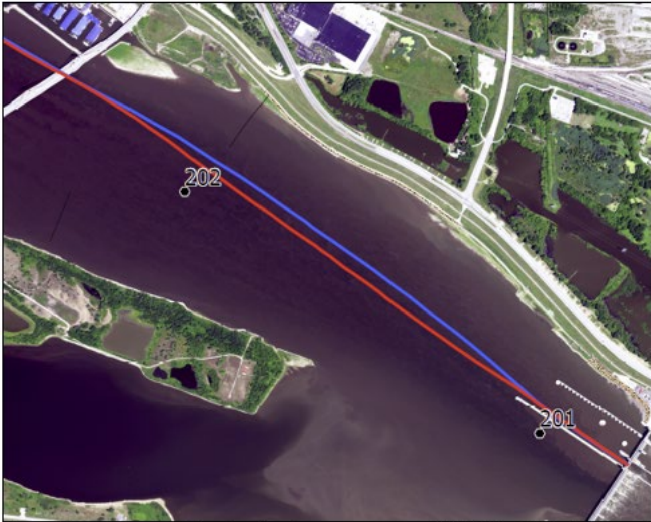
Figure 7: Sample image illustrating up bound vs. down bound tow movements at Melvin Price L&D. In this image, down bound tow paths are depicted by the blue line while the up bound paths are depicted by the red line. This is a sample illustration showing that regardless of direction of travel, vessels don't always use the same path of transit.
