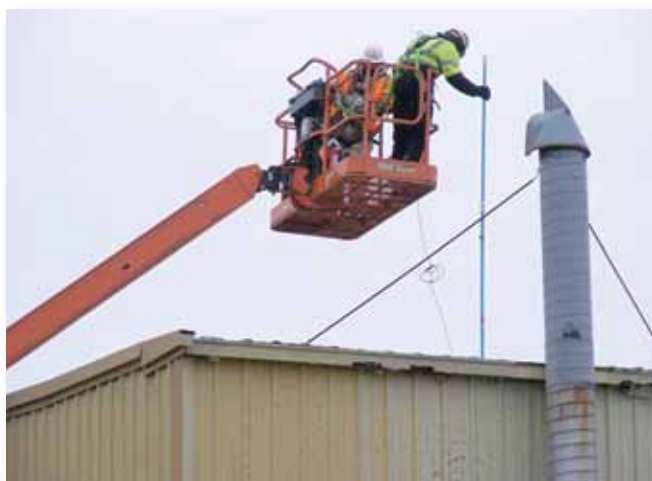
Sampling Futura property for radioactive contamination
