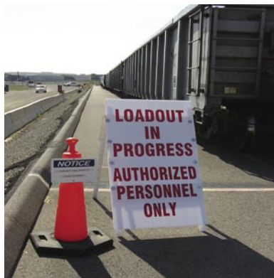
Loadout sign warns of danger during rail load operations.
