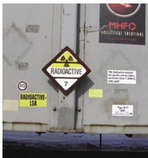
Placards, or signs, posted on the railcar help communicate the contents held by the railcar.
