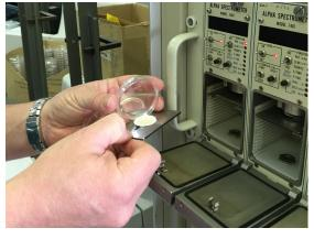
Technicians mount isolated thorium on a filter and insert it into the alpha spectrometer. This step tests for radium, thorium or uranium alpha particles in samples.
