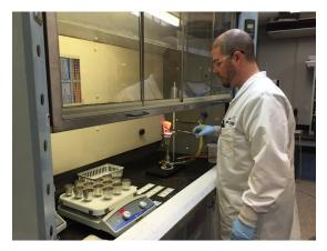
Here, a specially trained laboratory technician separates thorium from other isotopes in a sample so that thorium alone can be measured by alpha spectroscopy.
