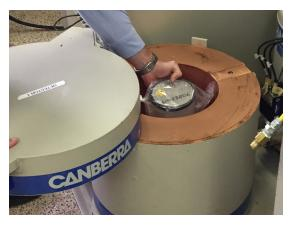
Here, a technician loads a soil sample into a gamma spectrometer. The instrument detects gamma rays emitted from the sample, identifies the isotopes within the sample and measures them.
