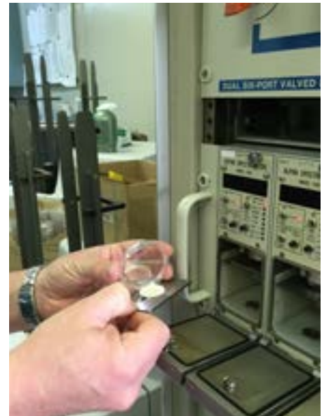
Alpha spectroscopy is used to analyze each sample's individual radiological isotope.
