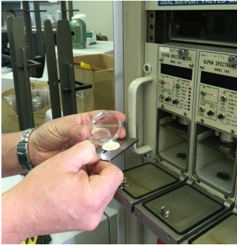
Alpha spectroscopy is used to analyze each sample’s individual radiological isotope.
