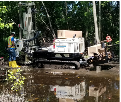
Drill rigs drill for soil samples quickly but getting them in place is not always easy because dense brush and woods and other obstructions limit access to many sampling locations.
