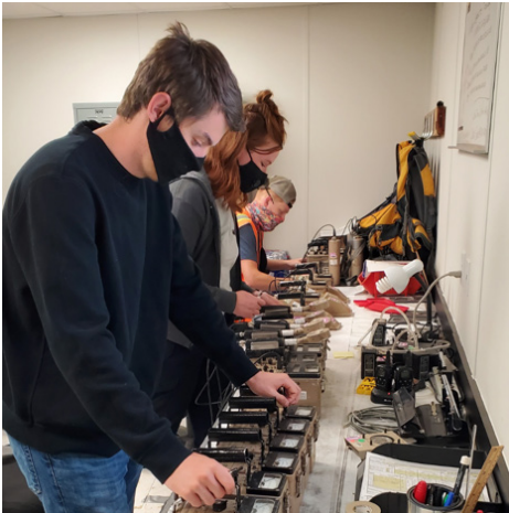
The FUSRAP radiological survey team checks their instruments’ calibrations daily. This step is necessary for data accuracy.
