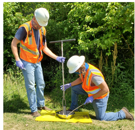
The FUSRAP team will collect soil samples from the surface to 6 feet or deeper. They collect samples manually most of the time but sometimes must use a drill rig for deeper samples.
