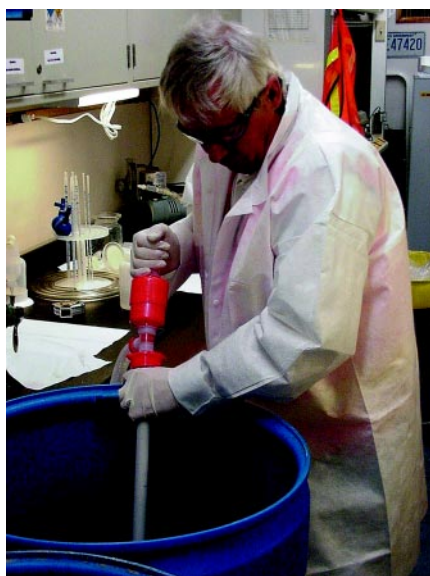
Crews carefully check excavation water before releasing it from the site to ensure it will not adversely affect local water bodies.
