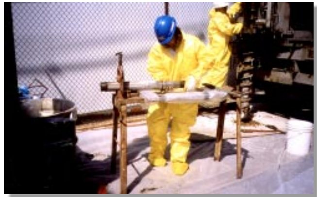
Systematically sampling Plants 1 and 6 will establish the excavation area and remediation volumes. The laborer shown here is working with a recently drilled soil sample.
