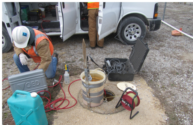
Groundwater monitoring wells are valuable for testing water quality and detecting contaminants of concern.
