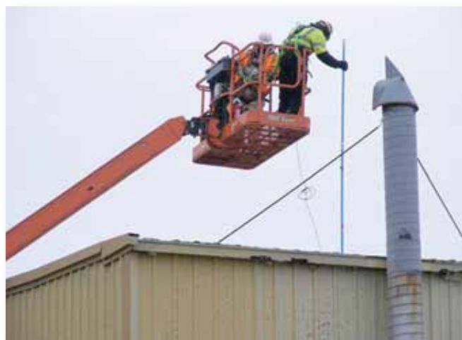
Sampling Futura property for radioactive contamination
