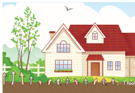
Radon gas filters up from soil and rocks everywhere. Only soil about 1-foot under or around a building affects its radon levels
