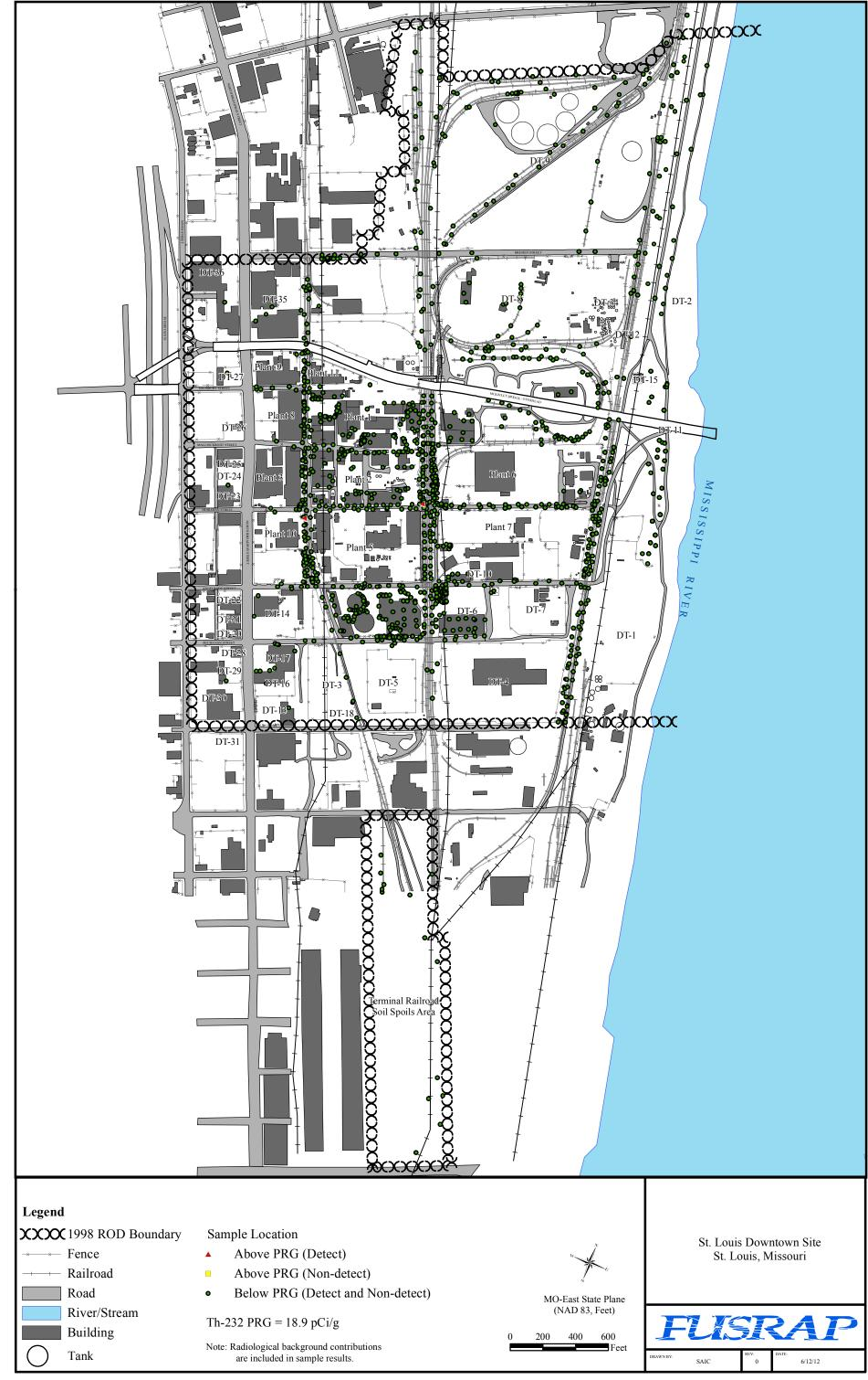
Figure C-7. Distribution of Th-232 Exceeding the PRG in Inaccessible Soil
