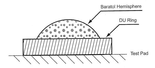
Figure 4. Diagrammatic Vertical Cross-Section of 'Hydroshot' Components.
