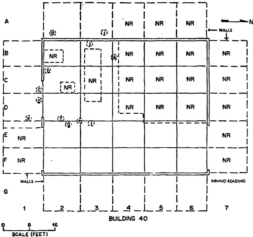
Fig. 7. Points on floor and lower walls in Building 40 where directly measured beta-gamma dose rates or alpha contamination levels exceeded background values (readings obtained at points "a" through "i" are given in Table 5).
