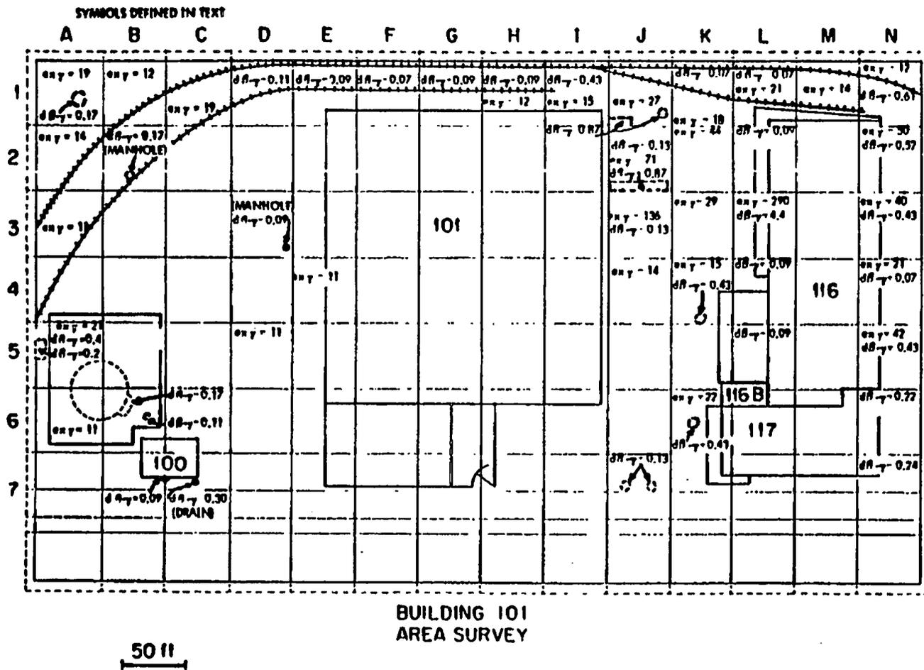
Fig. 38. Radiological measurements in survey blocks in area around Building 101. (See "Interpretation of Data" section on page 19 of text for explanation of symbols. The absence of numbers in survey blocks indicates that background levels were observed within that block.)
