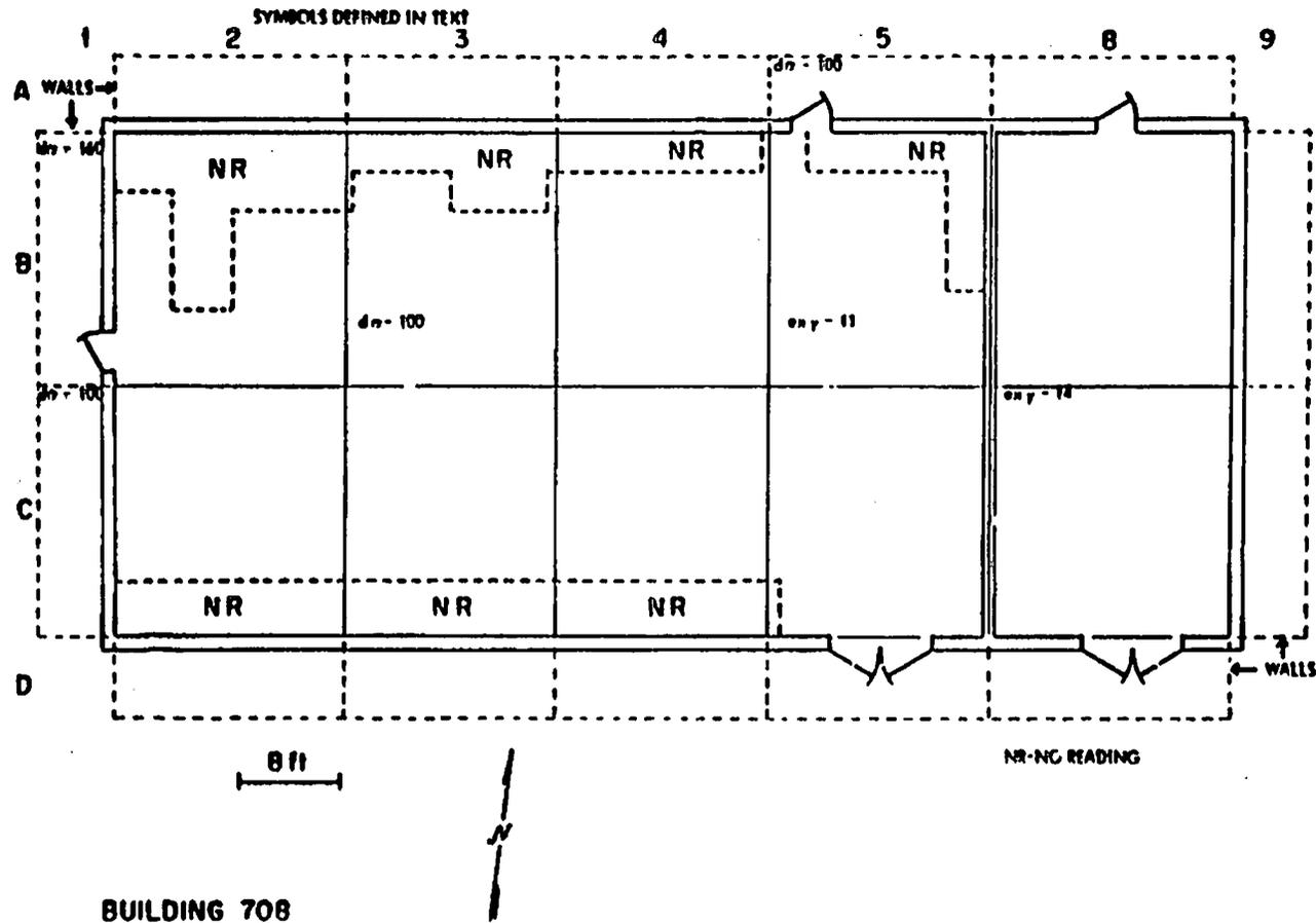
Fig. 34. Radiological measurements in survey blocks in Building 708. (See "Interpretation of Data" section on page 19 of text for explanation of symbols. The absence of numbers in survey blocks indicates that background levels were observed within that block.)
