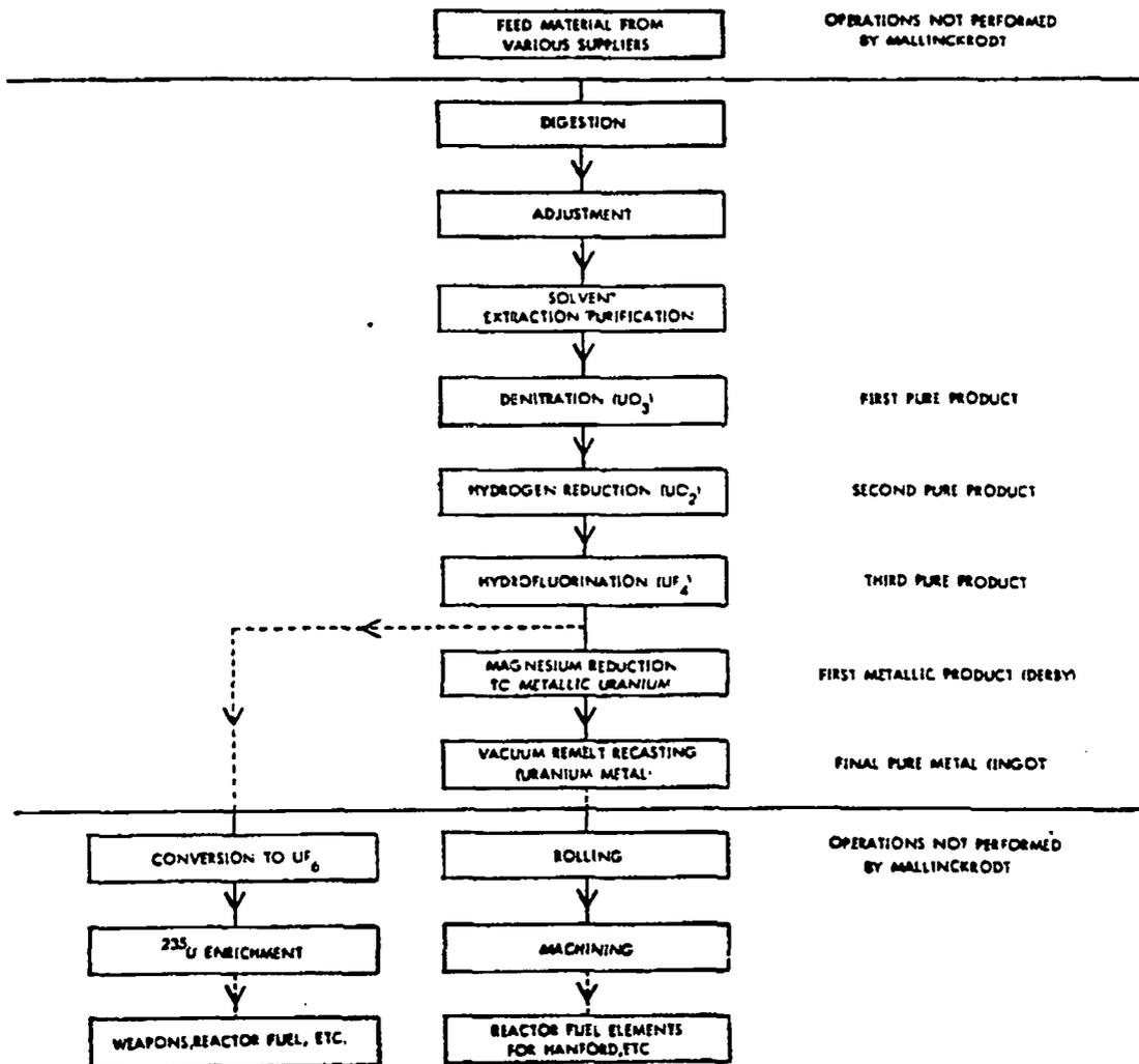
Fig. 2. Flow diagram of uranium refining process conducted at Mallinckrodt.
