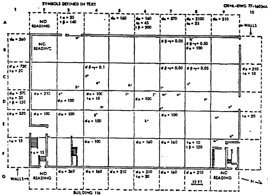
Fig. 15. Radiological measurements in survey blocks in main part of Building 116 (measurements at points indicated by lower-case letters are given in Table 16). (See "Interpretation of Data" section on page 19 of text for explanation of symbols. The absence of numbers in survey blocks indicates that background levels were observed within that block.)
