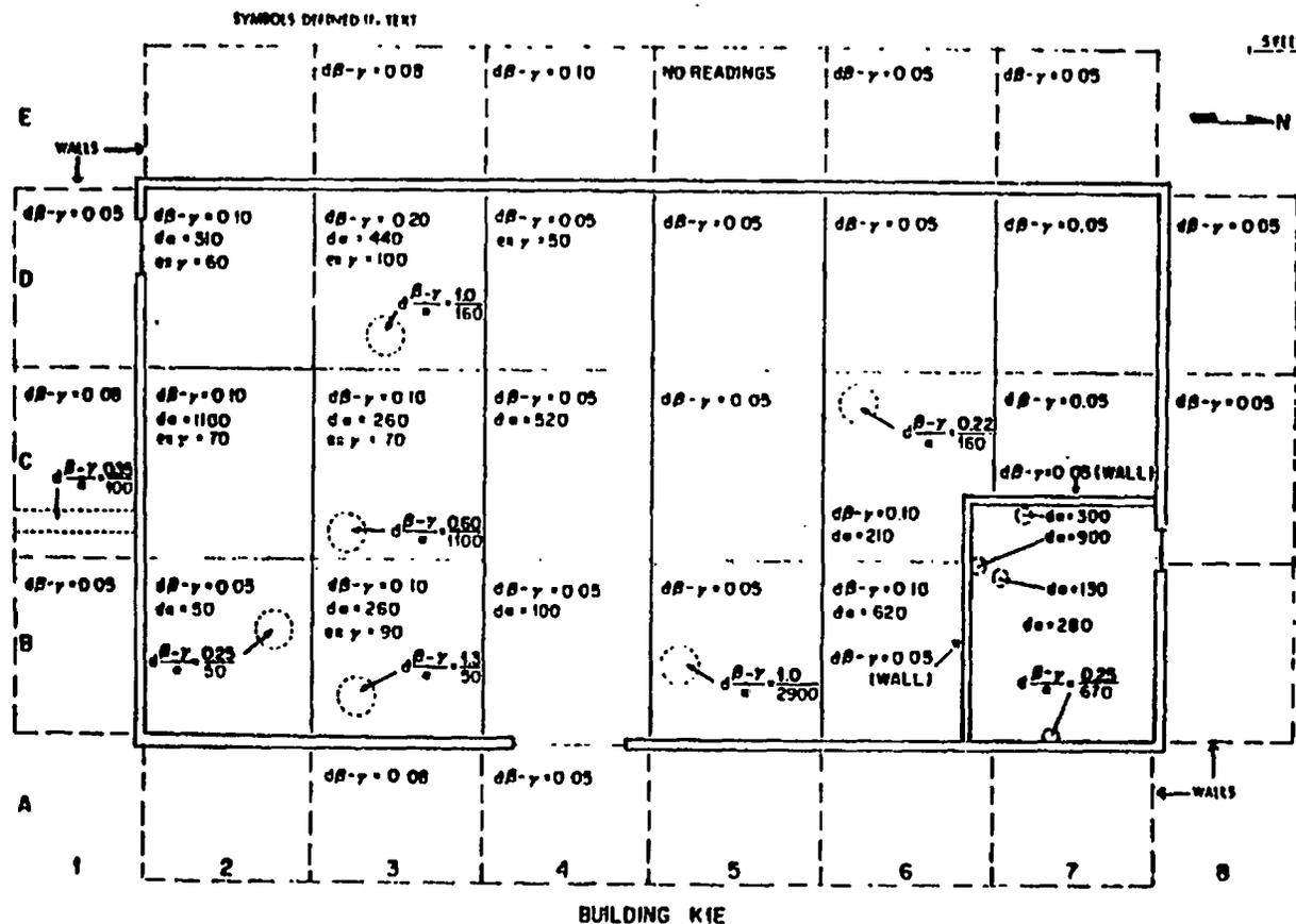
Fig. 3. Radiological measurements in survey blocks in Building K1E. (See "Interpretation of Data" section on page 19 of text for explanation of symbols. The absence of numbers in survey blocks indicates that background levels were observed within that block.)
