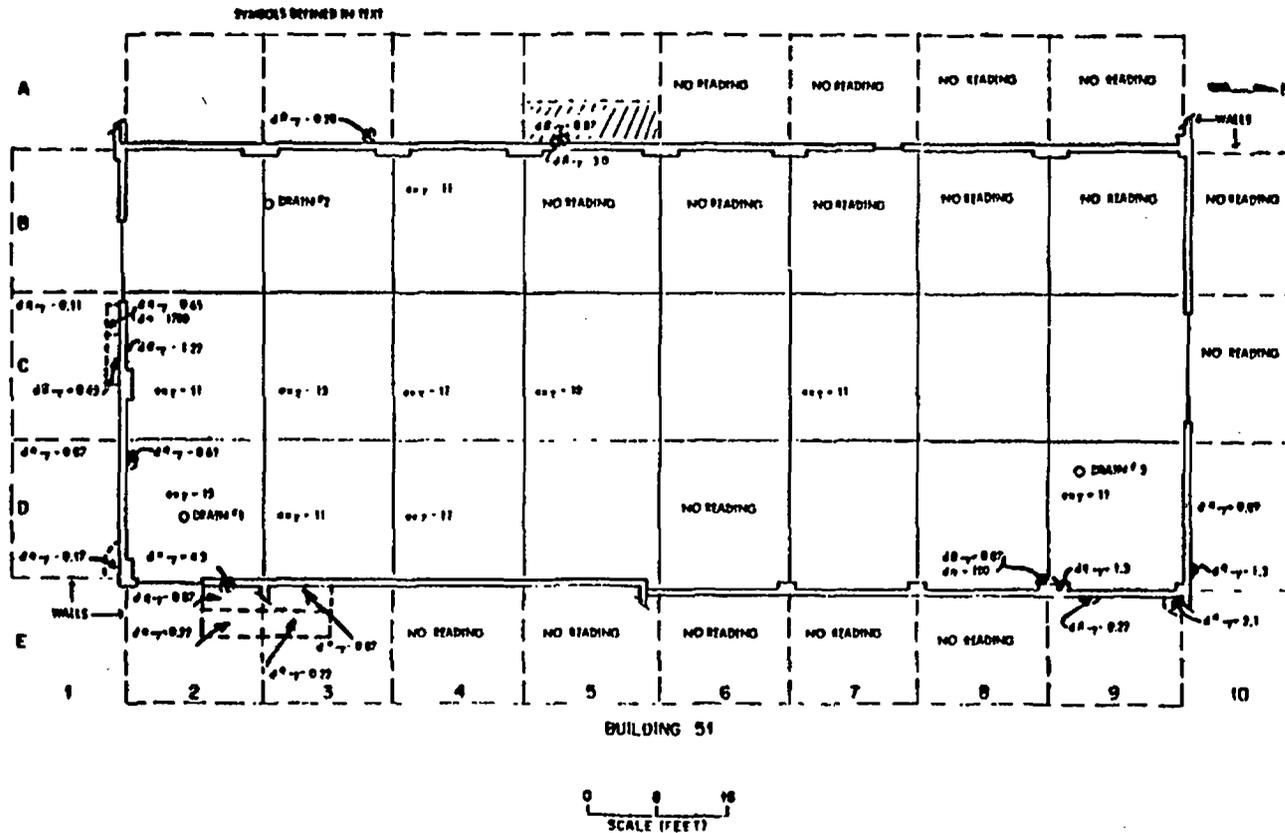
Fig. 9. Radiological measurements in survey blocks in Building 51 (measurements made in drains are given in Table 7). (See "Interpretation of Data" section on page 19 of text for explanation of symbols. The absence of numbers in survey blocks indicates that background levels were observed within that block.)
