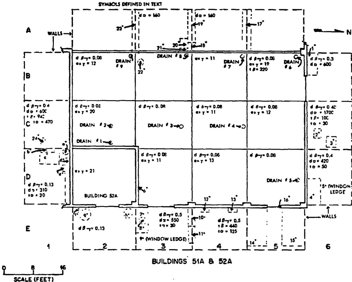
Fig. 11. Radiological measurements in survey blocks in Buildings 51A and 52A (measurements in areas marked with asterisks are given in Tables 11 and 14; measurements made in drains are given in Table 7). (See "Interpretation of Data" section on page 19 of text for explanation of symbols. The absence of numbers in survey blocks indicates that background levels were observed within that block.)
