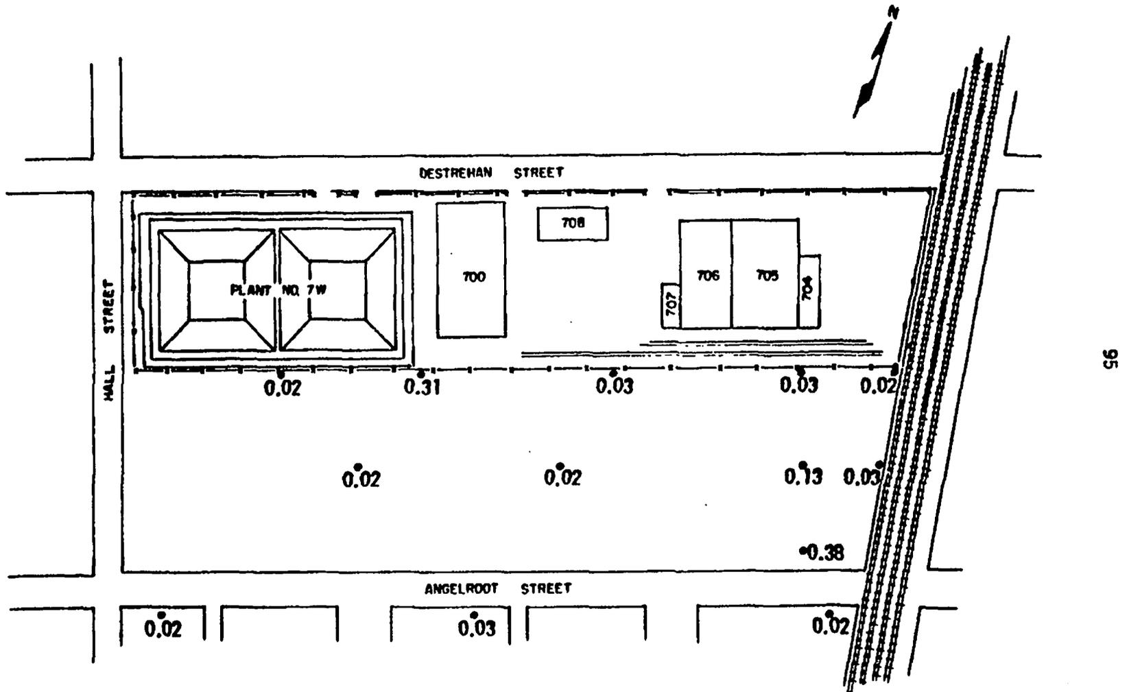
Fig. 41. Beta-gamma dose rates (mrad/h) at 1 cm from the surface in randomly selected locations south of Buildings 700, 704, 705, 706, 707, and 708.
