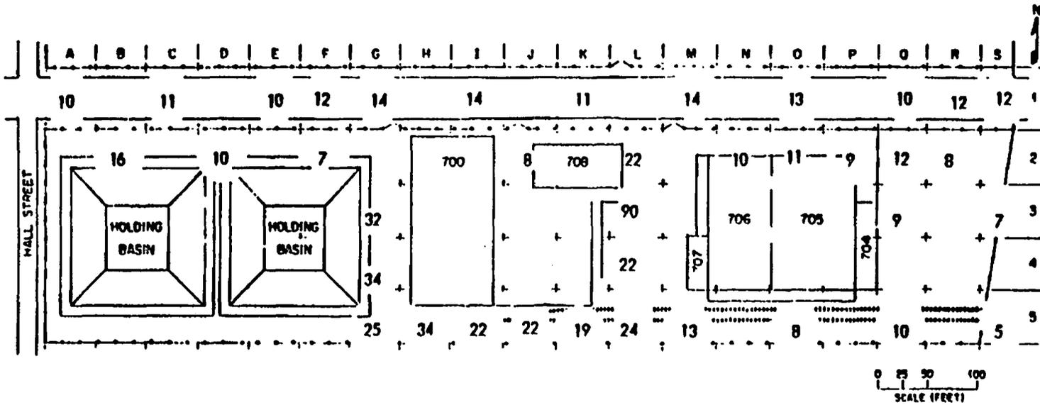
Fig. 40. External gamma radiation levels ( $\mu\text{R/h}$ ) at 1 m above surface in survey blocks around Buildings 700, 704, 705, 706, 707, and 708.
