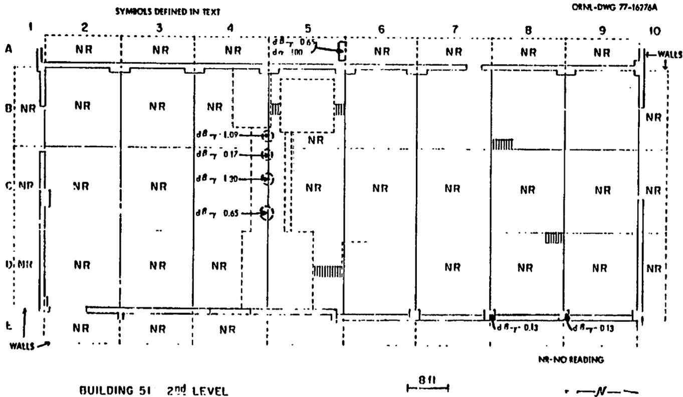
Fig. 10. Radiological measurements on second level of Building 51. (See "Interpretation of Data" section on page 19 of text for explanation of symbols. The absence of numbers in survey blocks indicates that background levels were observed within that block.)
