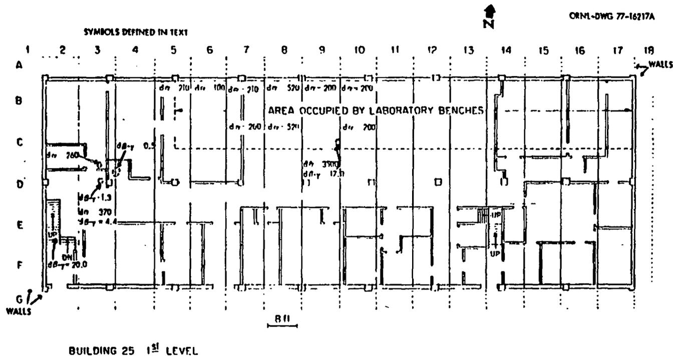
Fig. 4. Radiological measurements in survey blocks in Building 25, first level. (See "Interpretation of Data" section on page 19 of text for explanation of symbols. The absence of numbers in survey blocks indicates that background levels were observed within that block.)
