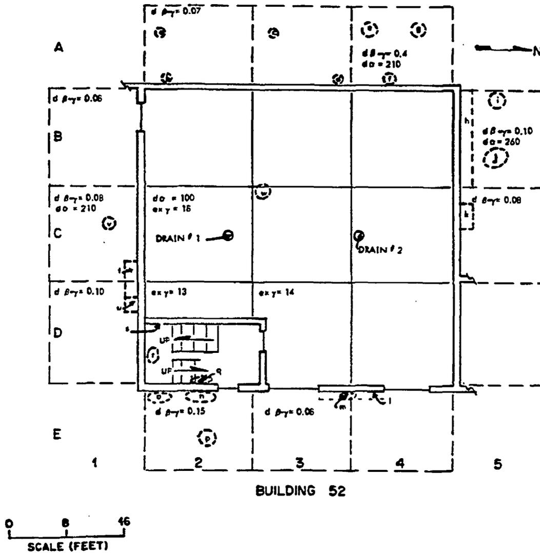
Fig. 12. Radiological measurements in survey blocks in Building 52 (measurements in areas indicated by lower-case letters are given in Table 15; measurements made in drains are given in Table 7). (See "Interpretation of Data" section on page 19 of text for explanation of symbols. The absence of numbers in survey blocks indicates that background levels were observed within that block.)
