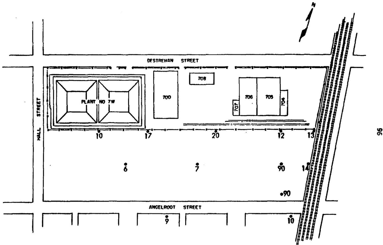
Fig. 42. External gamma radiation levels ( $\mu\text{R/h}$ ) at 1 m above the surface in randomly selected locations south of Buildings 700, 704, 705, 706, 707, and 708.
