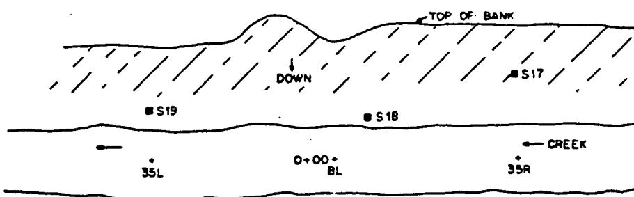
Fig. 3. Locations of surface soil samples taken at Latty Avenue (LM001) between 0+00, BL and 2+00, BL.
