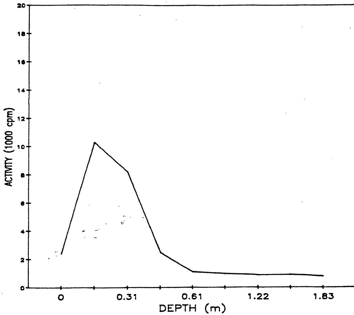
Fig. A.73. Gamma profile of auger hole 73.
