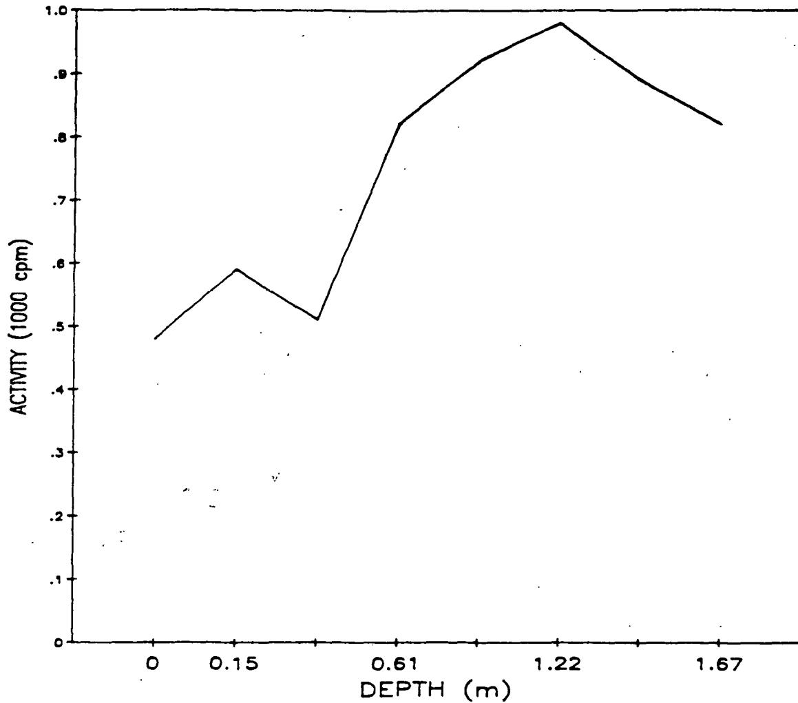
Fig. A.29. Gamma profile of auger hole 29.
