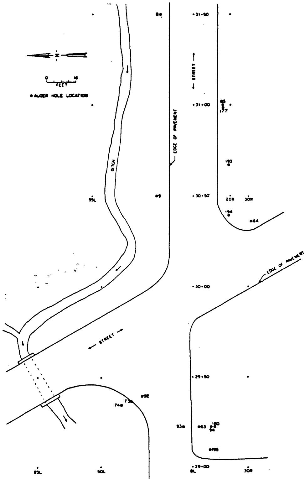
Fig. 28. Locations of auger holes at Latty Avenue (LM001) between 29+00, BL and 31+50, BL.
