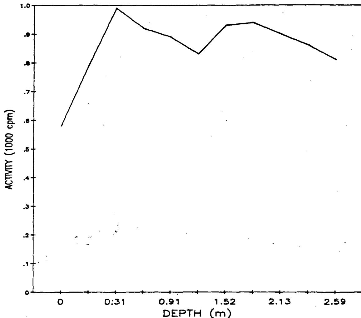
Fig. A.7. Gamma profile of auger hole 7.
