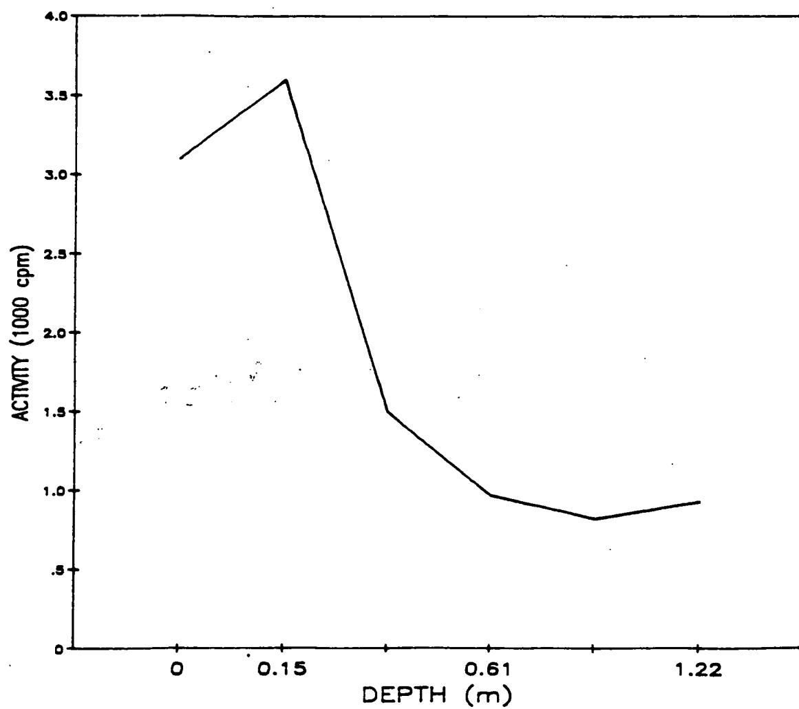
Fig. A.66. Gamma profile of auger hole 66.
