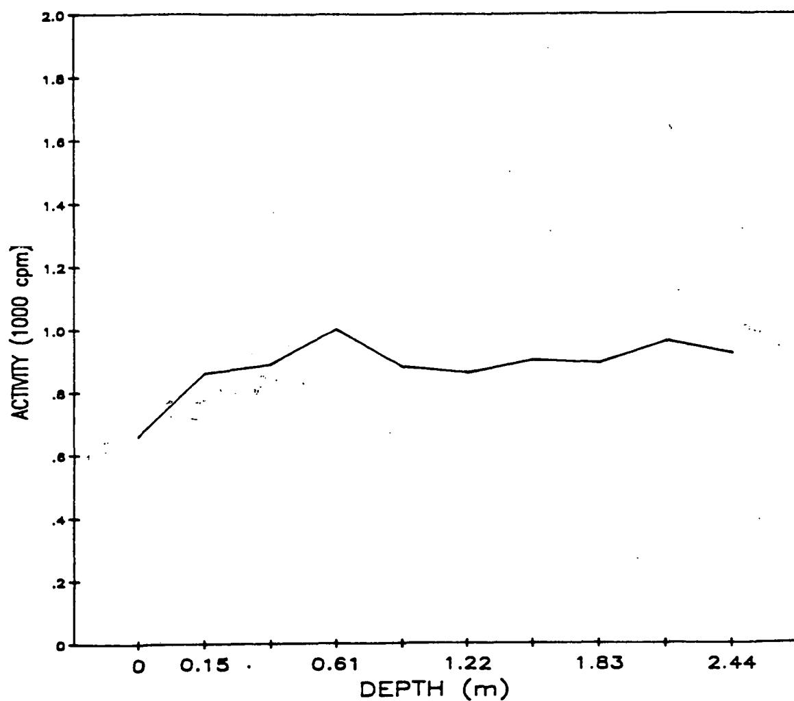
Fig. A.4. Gamma profile of auger hole 4.
