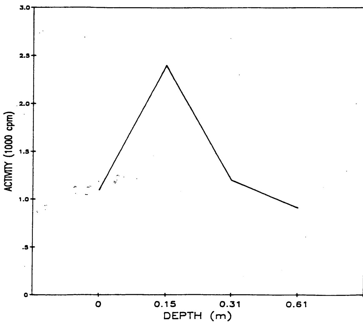
Fig. A.64. Gamma profile of auger hole 64.
