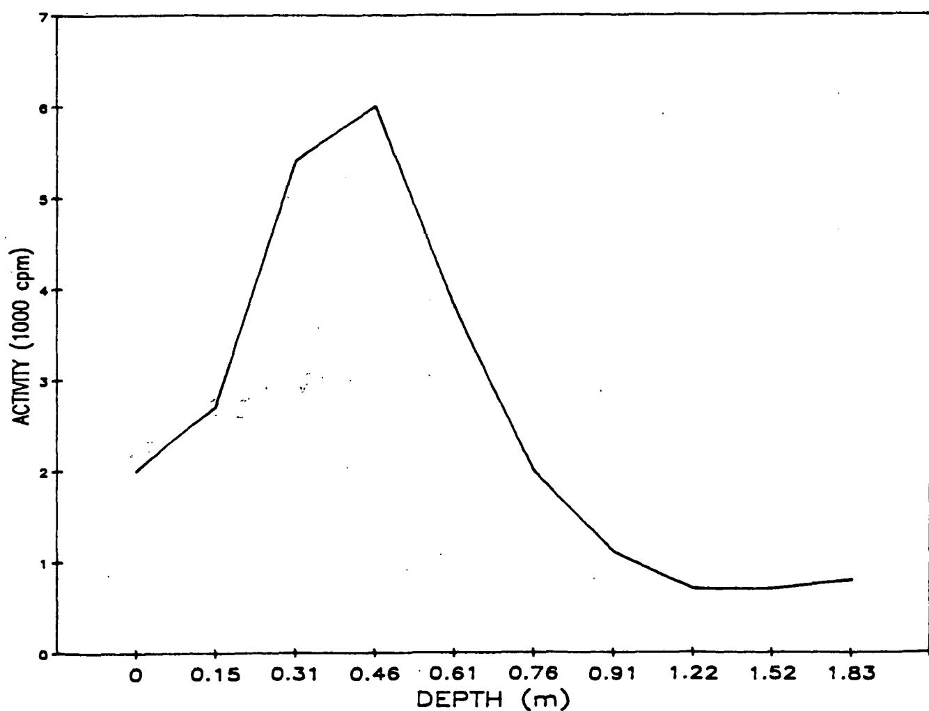
Fig. A.154. Gamma profile of auger hole 154.
