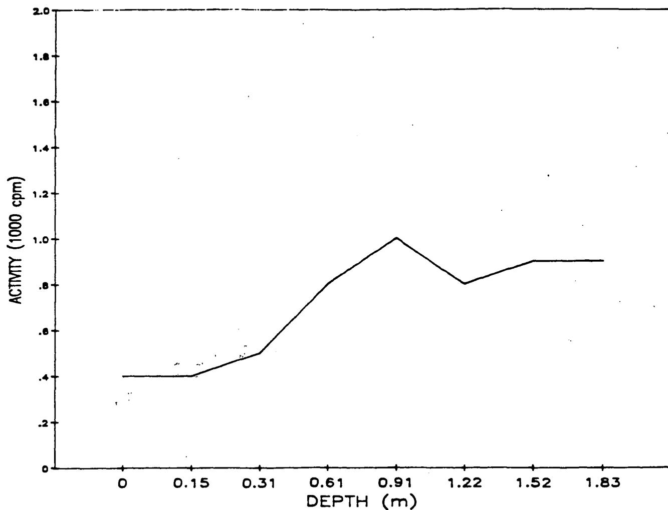
Fig. A.139. Gamma profile of auger hole 139.
