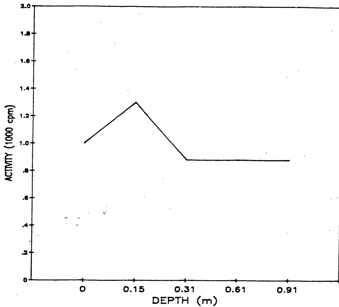
Fig. A.111. Gamma profile of auger hole 111.
