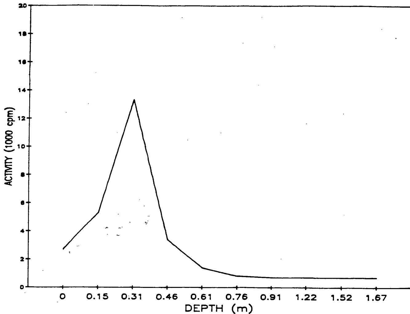
Fig. A.159. Gamma profile of auger hole 159.
