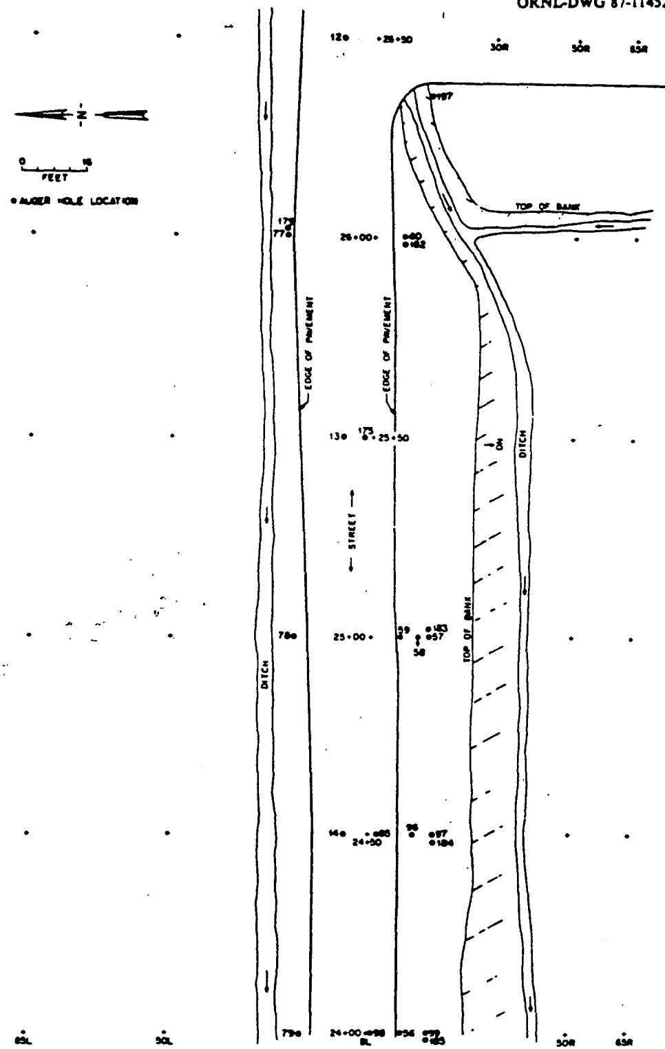
Fig. 26. Locations of auger holes at Latty Avenue (LM001) between 24+00, BL and 26+50, BL.
