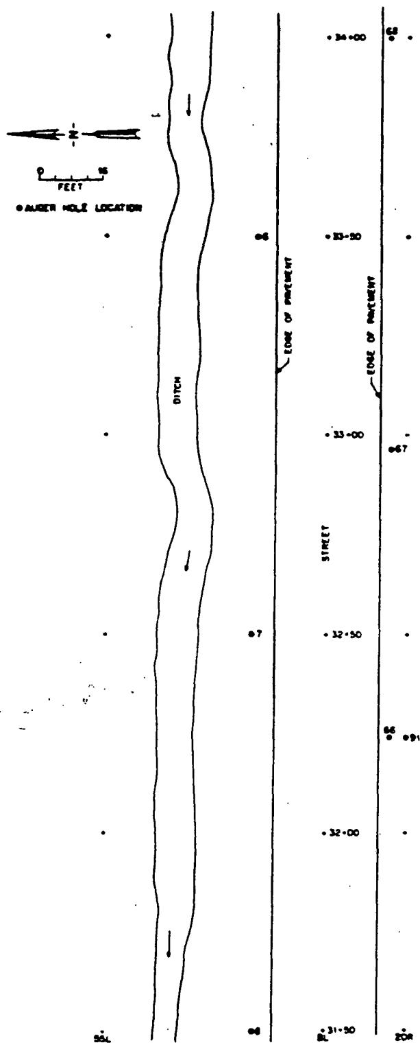
Fig. 29. Locations of auger holes at Latty Avenue (LM001) between 31+50, BL and 34+00, BL.
