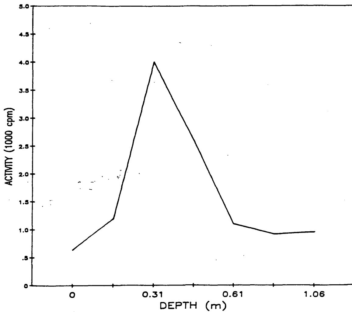
Fig. A.56. Gamma profile of auger hole 56.
