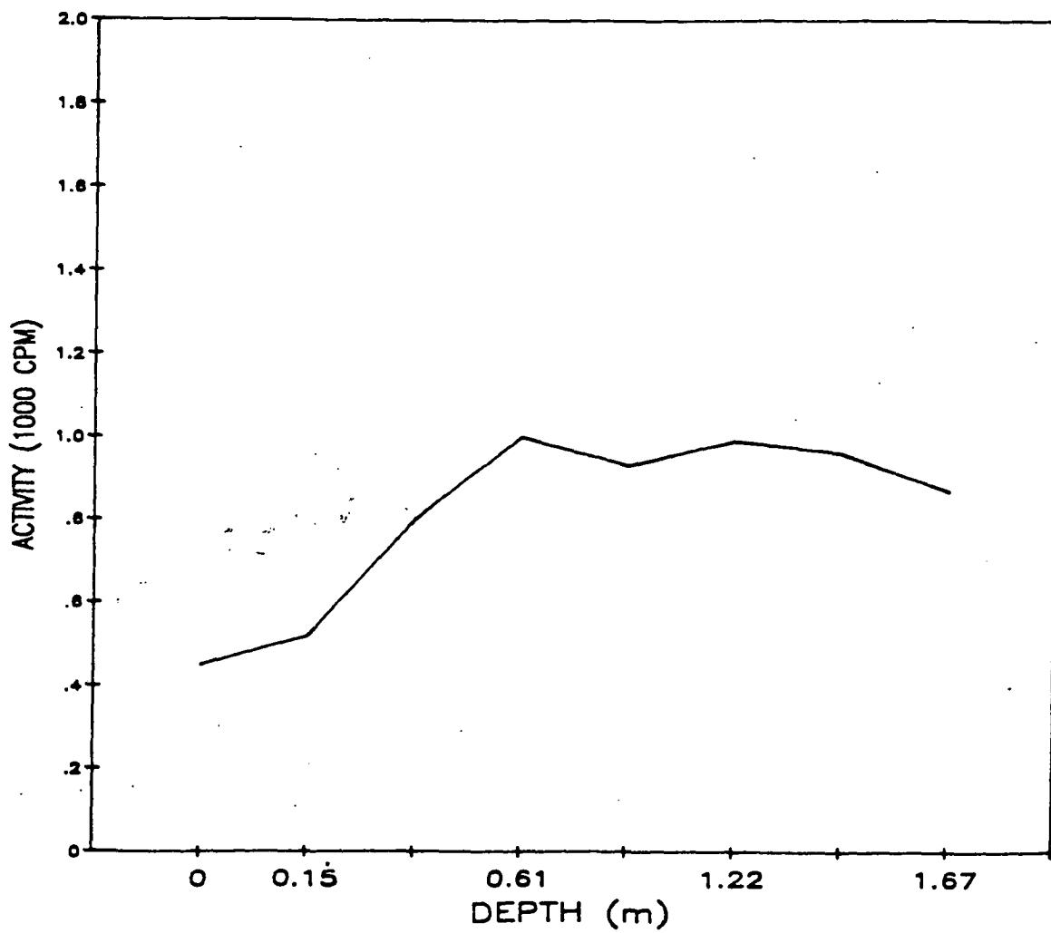
Fig. A.20. Gamma profile of auger hole 20.
