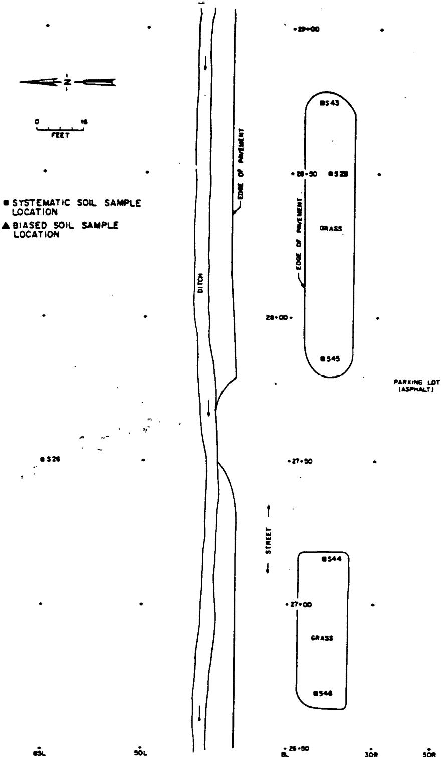
Fig. 14. Locations of surface soil samples taken at Latty Avenue (LM001) between 26+50, BL and 29+00, BL.
