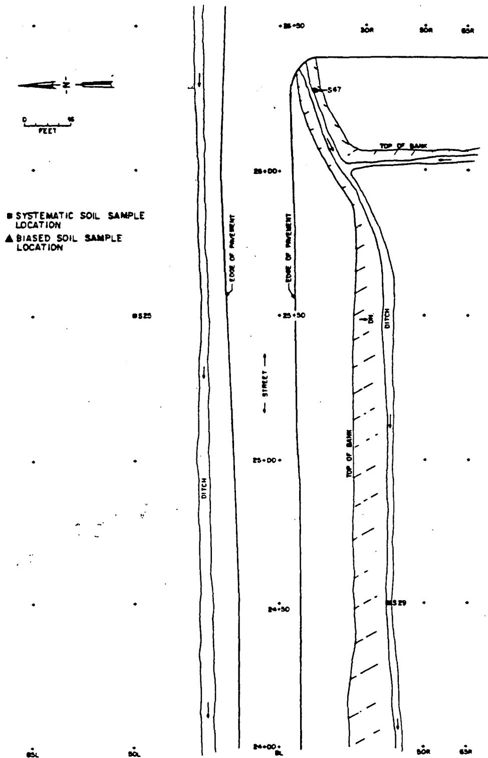
Fig. 13. Locations of surface soil samples taken at Latty Avenue (LM001) between 24+00, BL and 26+50, BL.
