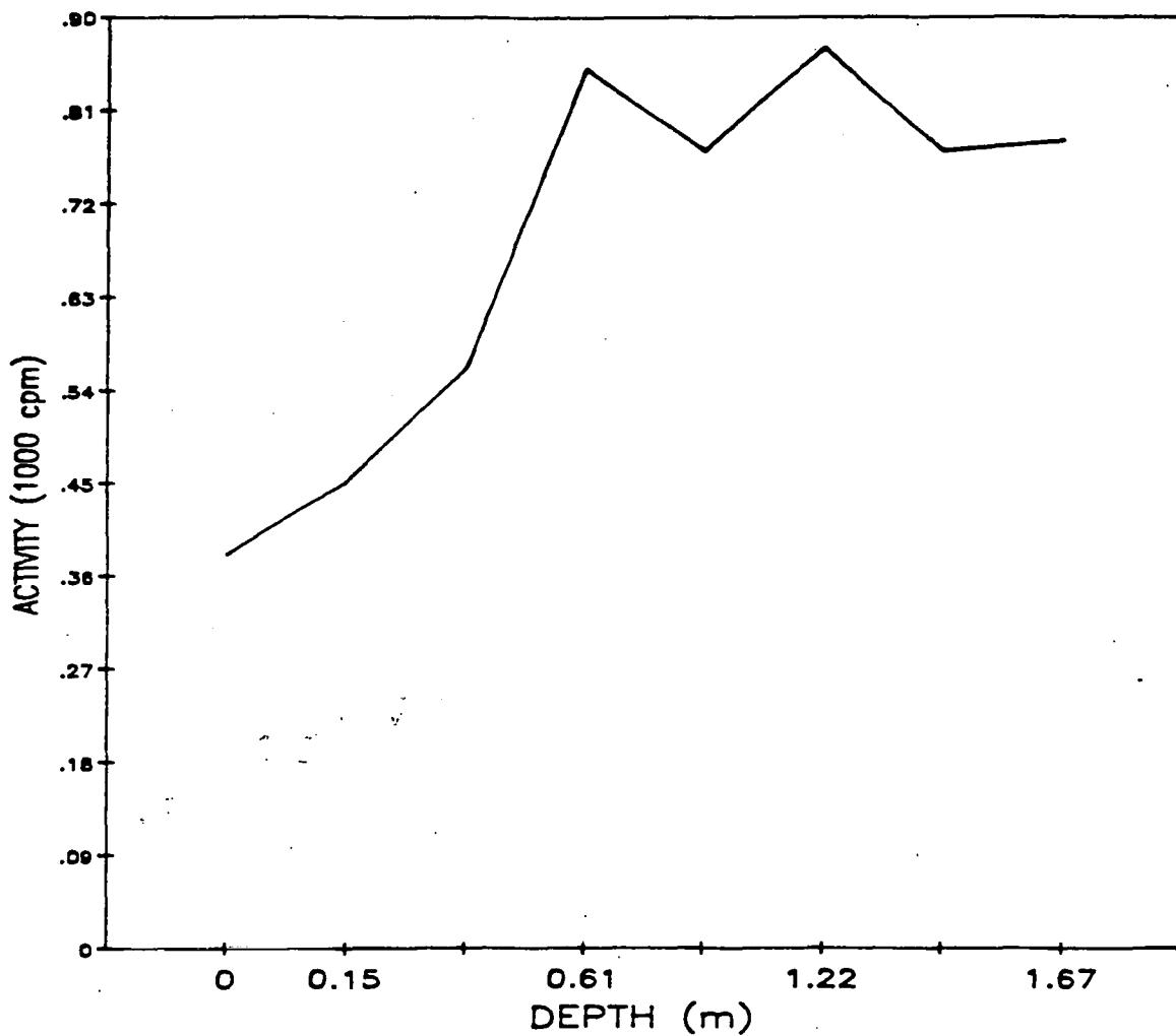
Fig. A.13. Gamma profile of auger hole 13.
