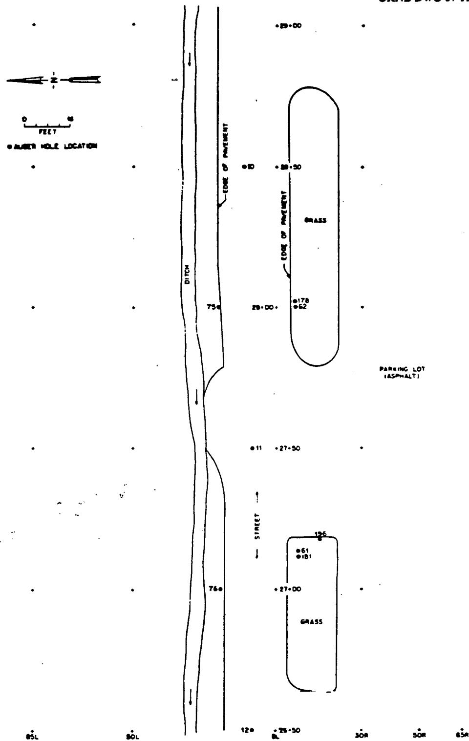
Fig. 27. Locations of auger holes at Latty Avenue (LM001) between 26 + 50, BL and 29 + 00, BL.
