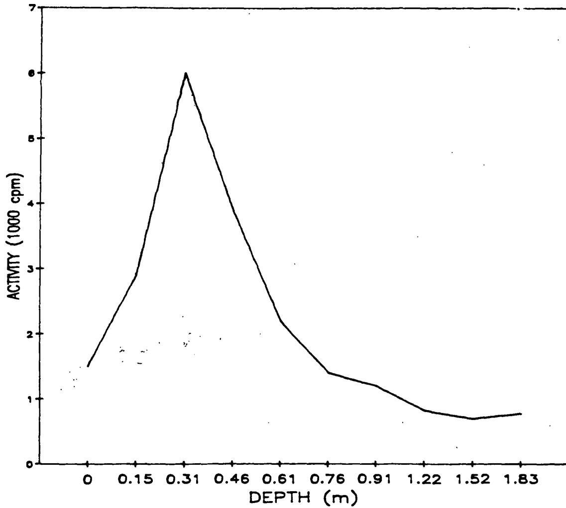
Fig. A.119. Gamma profile of auger hole 119.
