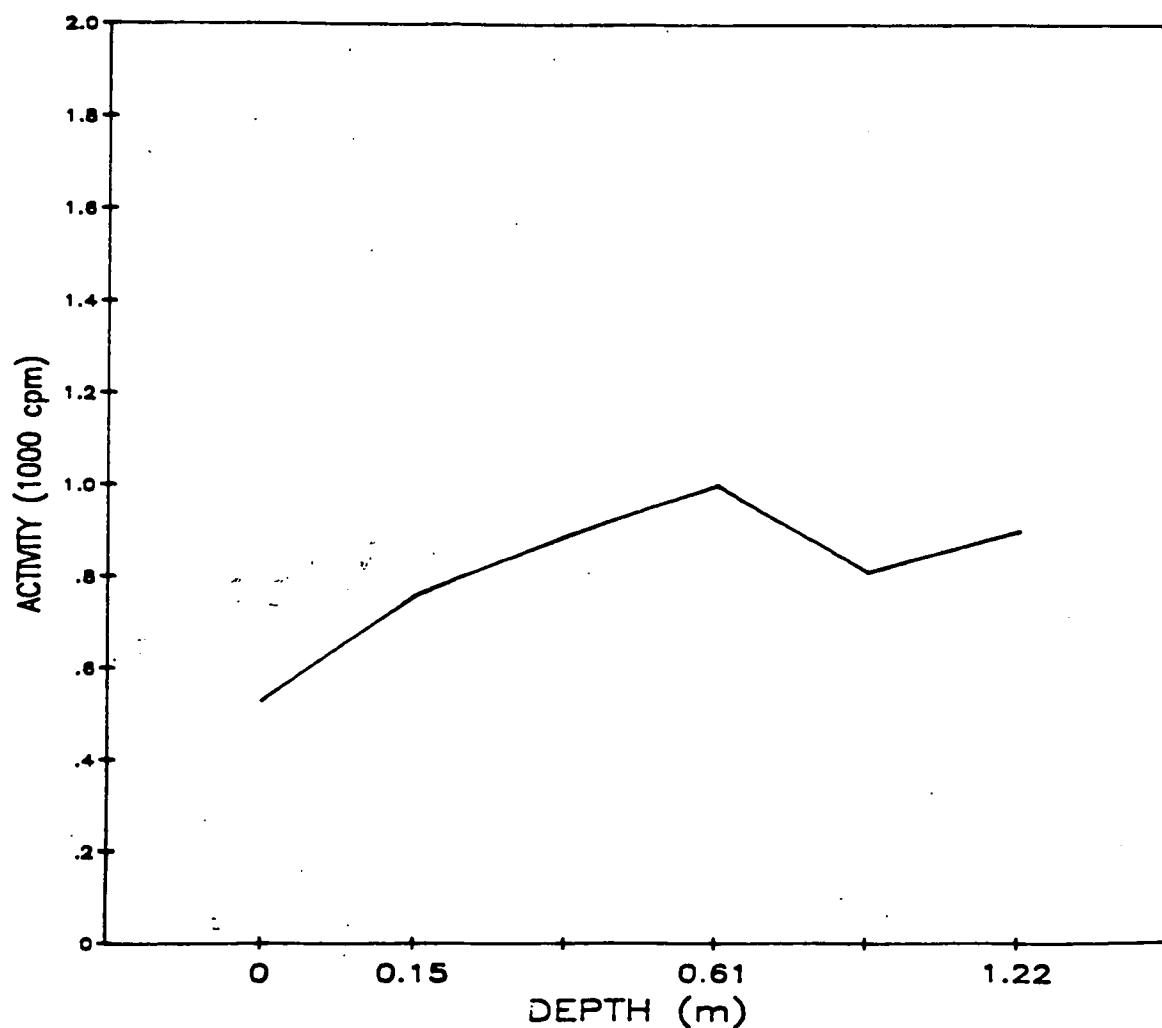
Fig. A.68. Gamma profile of auger hole 68.
