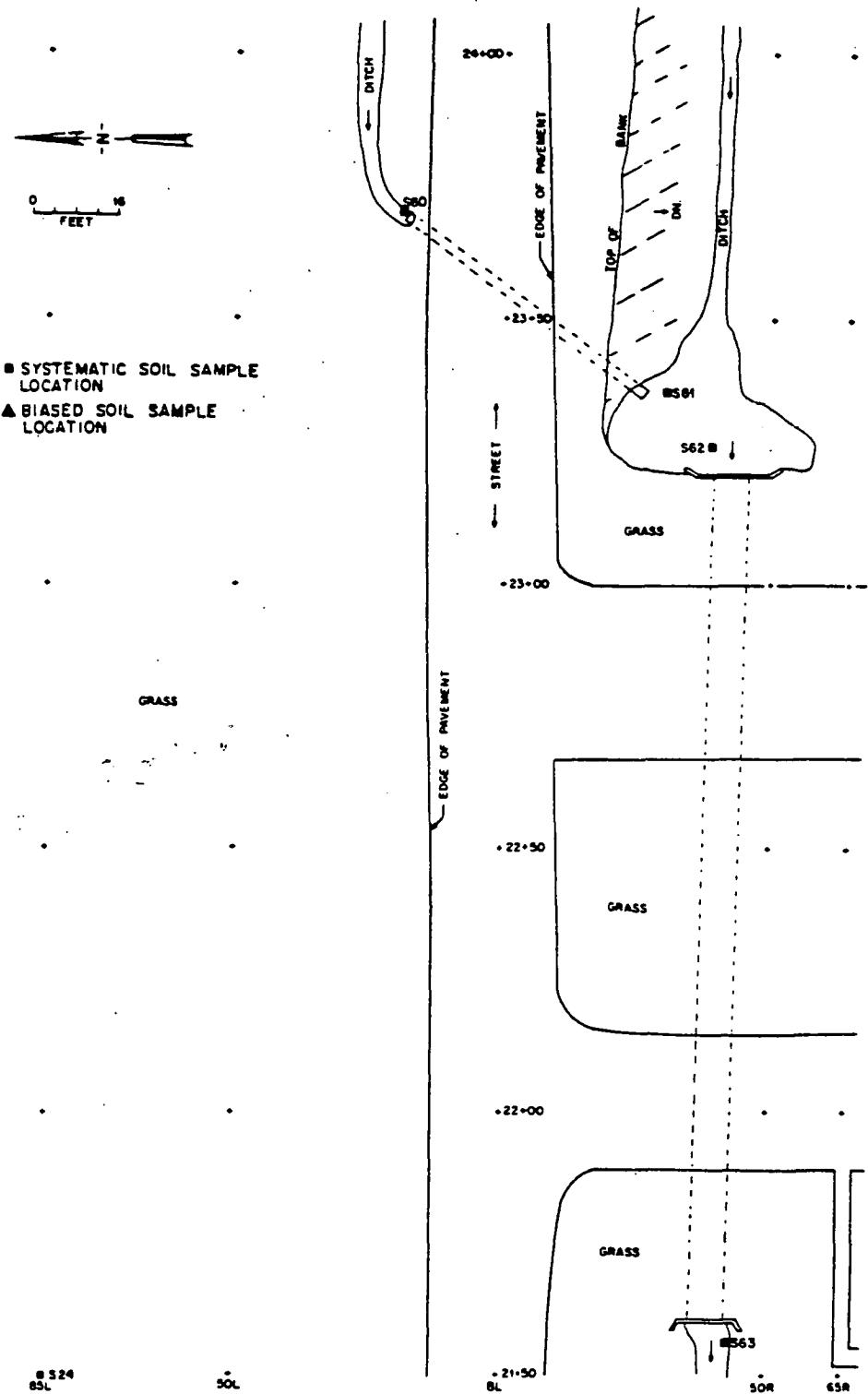
Fig. 12. Locations of surface soil samples taken at Latty Avenue (LM001) between 21+50, BL and 24+00, BL.
