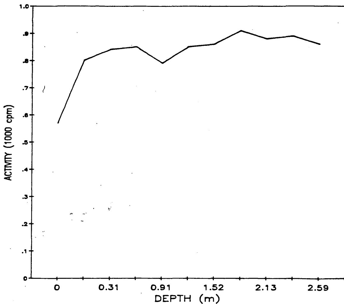
Fig. A.9. Gamma profile of auger hole 9.
