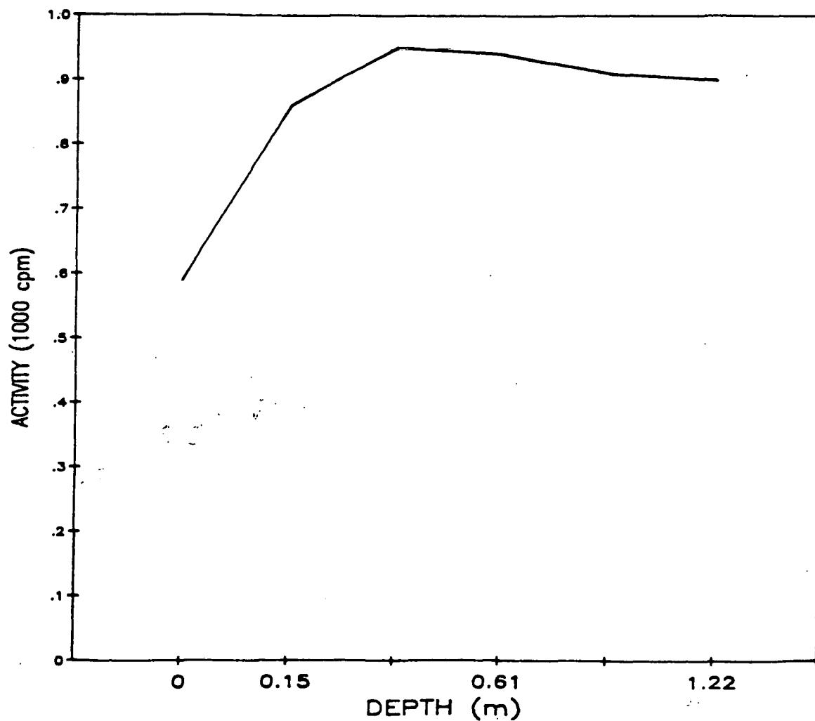
Fig. A.44. Gamma profile of auger hole 44.
