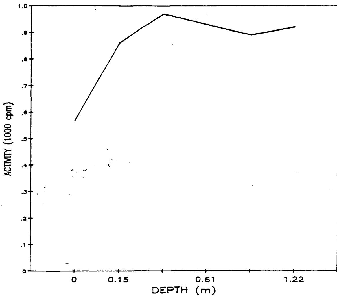
Fig. A.40. Gamma profile of auger hole 40.
