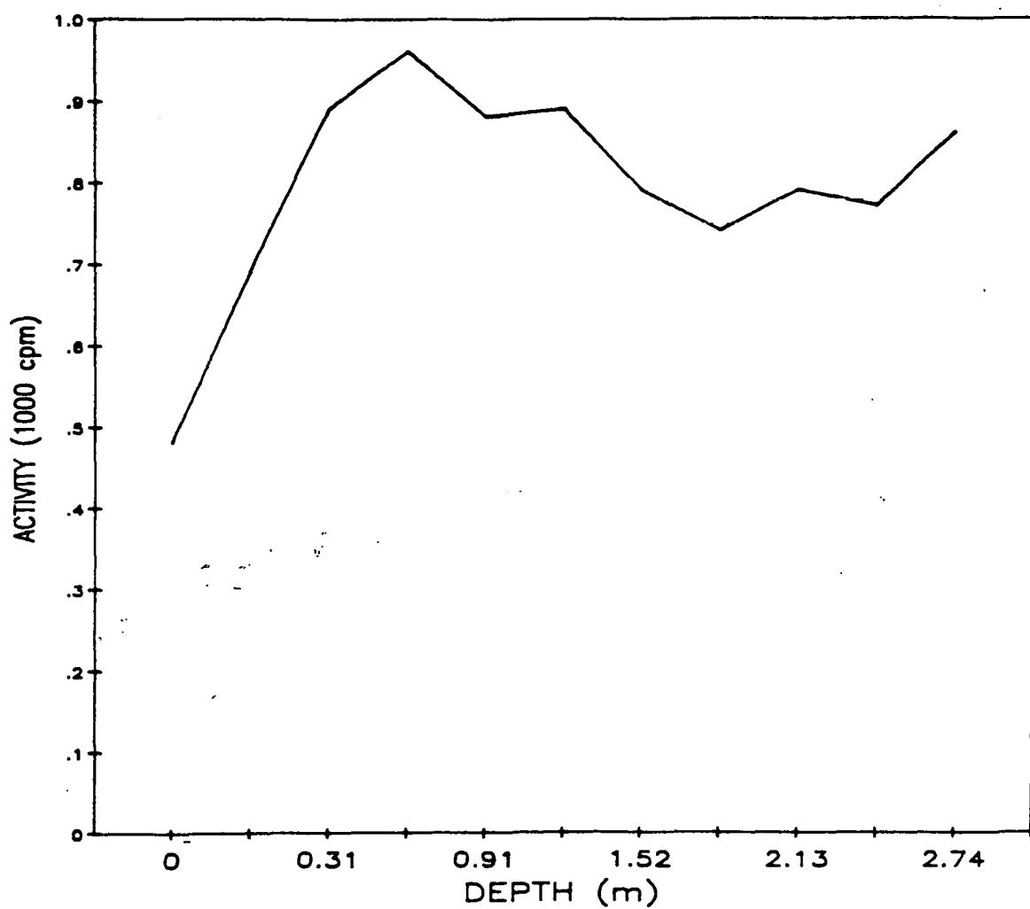
Fig. A.8. Gamma profile of auger hole 8.
