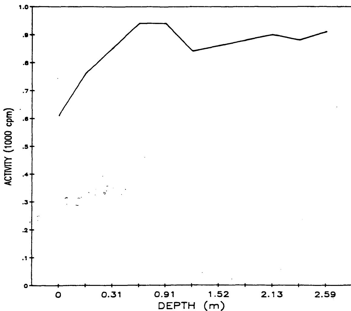
Fig. A.6. Gamma profile of auger hole 6.
