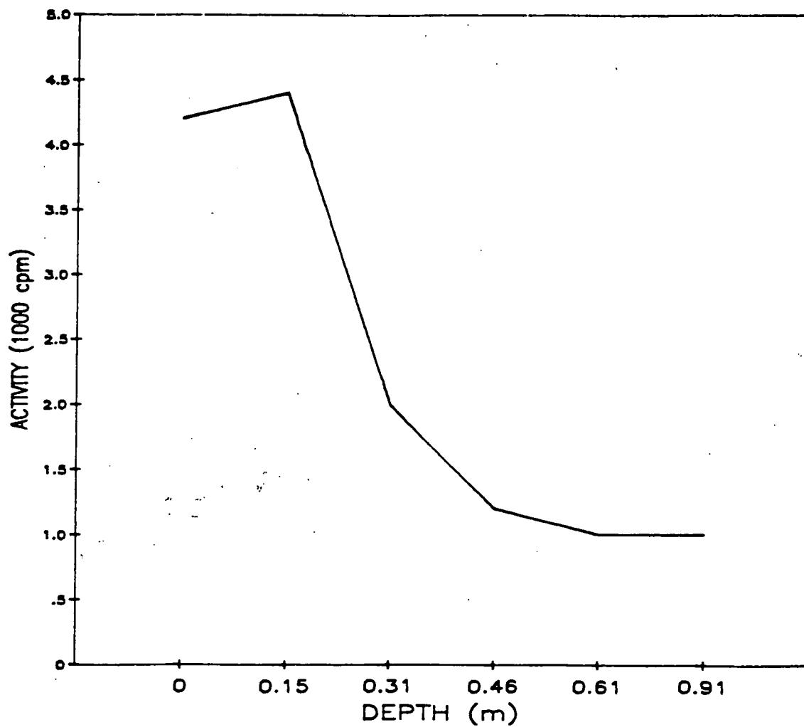
Fig. A.149. Gamma profile of auger hole 149.
