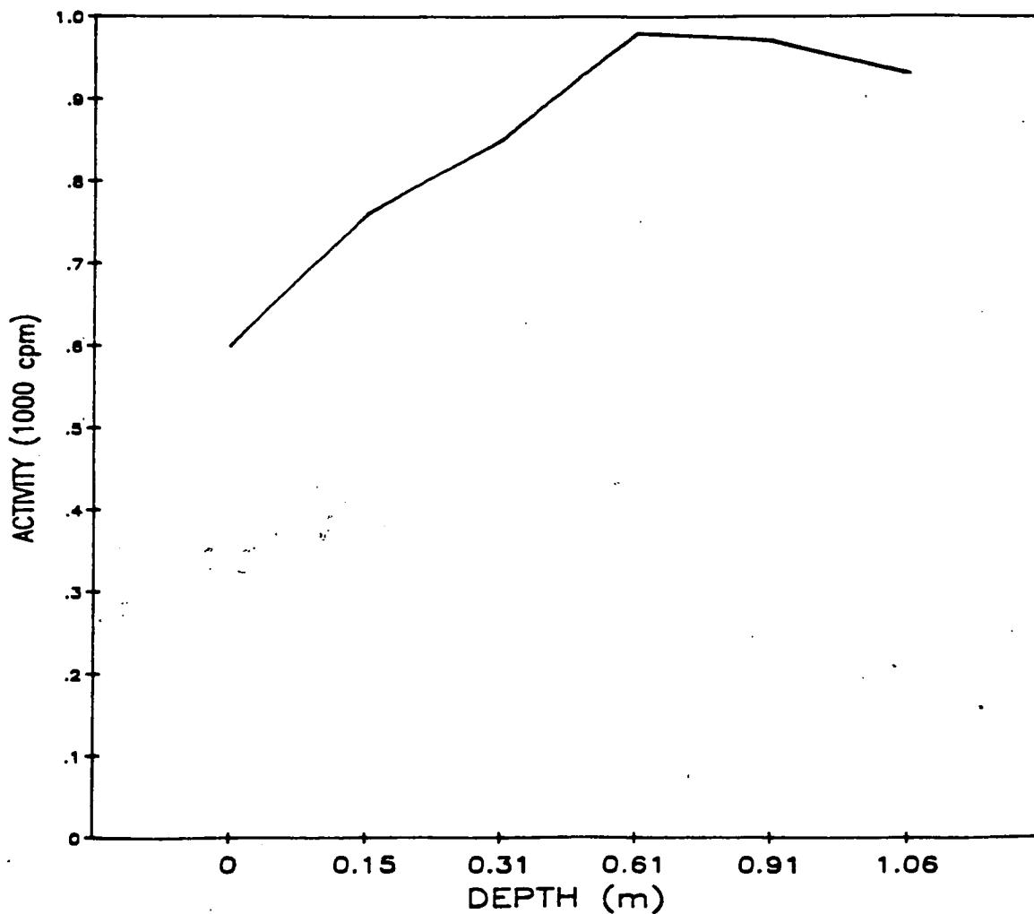
Fig. A.34. Gamma profile of auger hole 34.
