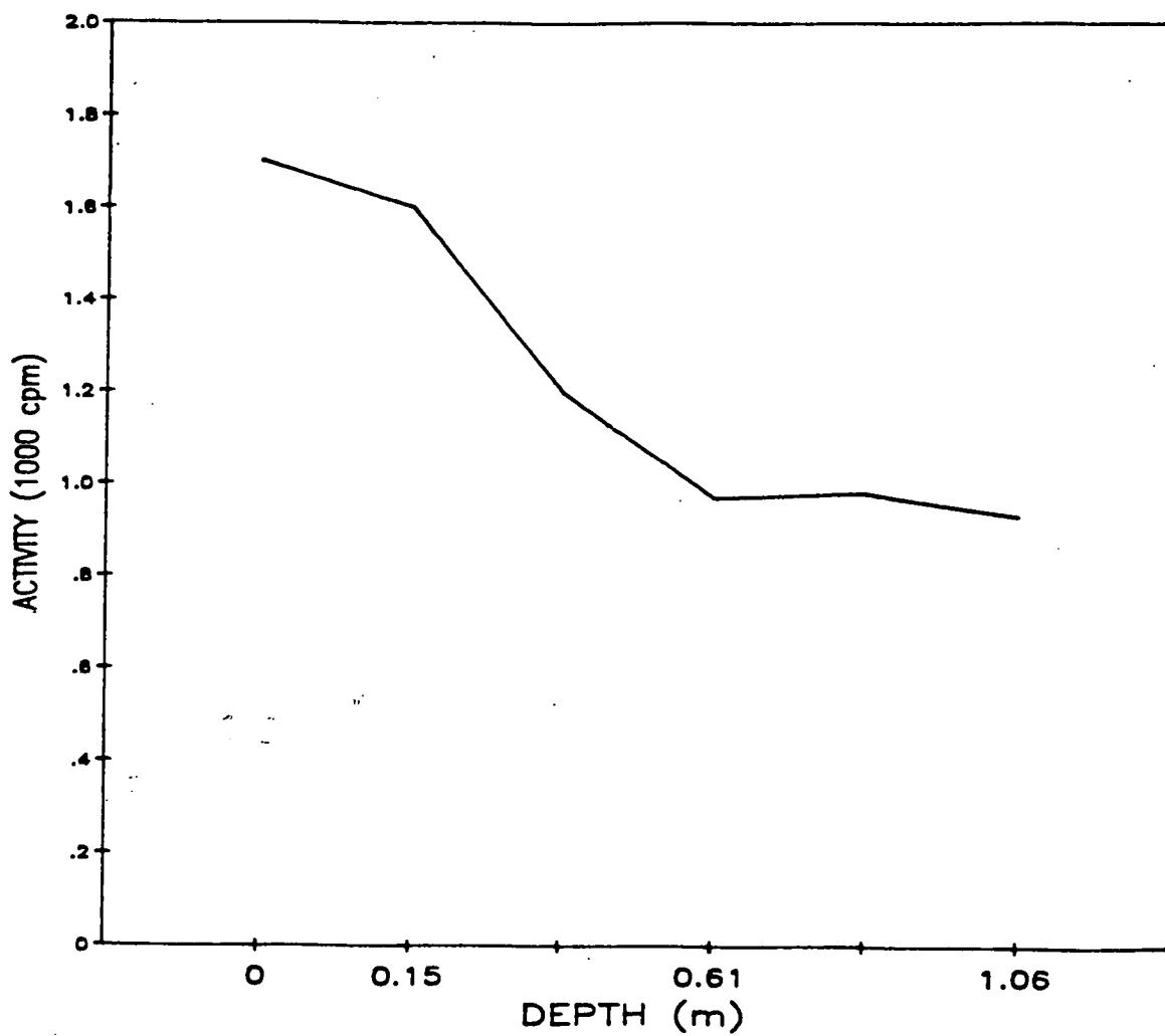
Fig. A.43. Gamma profile of auger hole 43.
