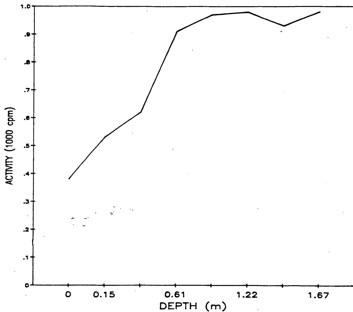
Fig. A.11. Gamma profile of auger hole 11.
