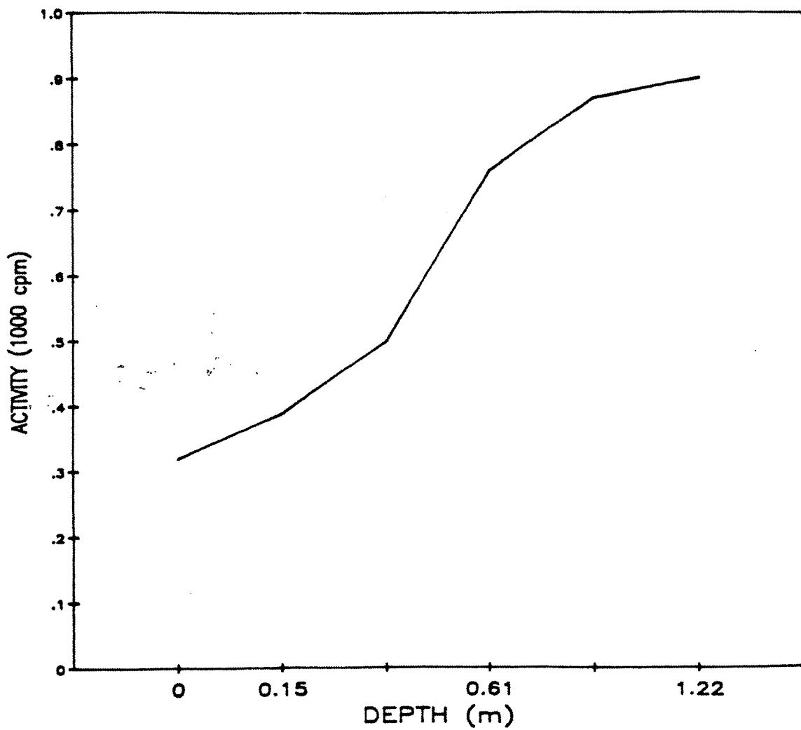
Fig. A.92. Gamma profile of auger hole 92.
