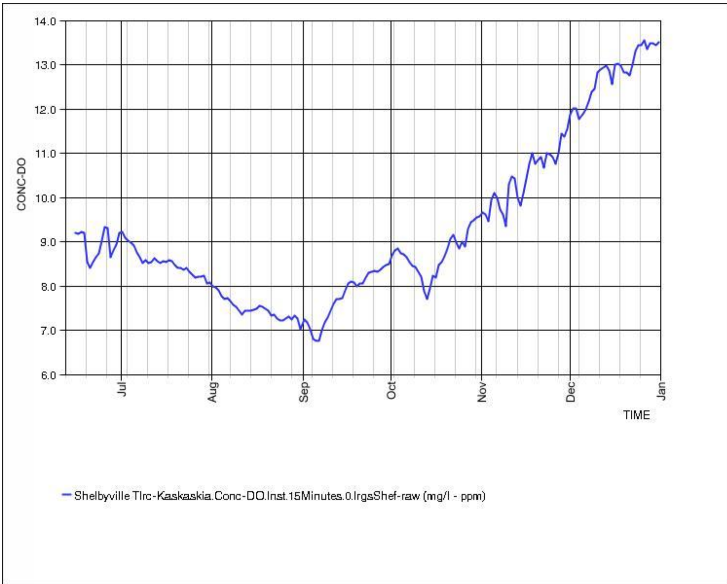
Dissolved Oxygen in spillway as monitored by remote sonde
