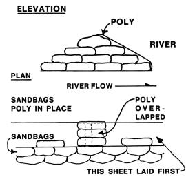
Polyethylene (poly) comes in rolls 20 ft by 100 ft (or 200 ft). It is used to wrap sandbag levees to prevent seepage. The poly should be placed on the downstream portion of the levee first, then worked upstream with a two- to three-foot overlap. There should be at least a two-foot overlap along the riverside toe and it must be anchored down with sandbags, both at the toe, and along the sideslopes.
