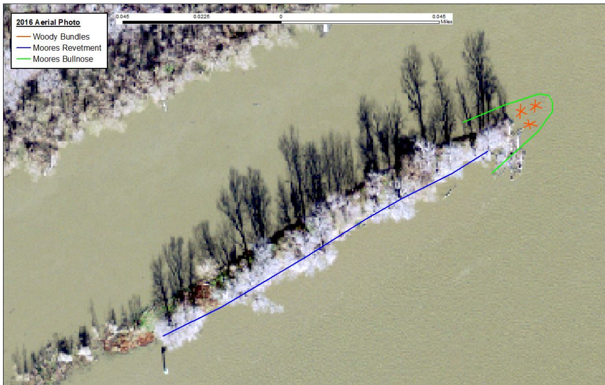
Figure 5. Recommended Mitigation Alternative: Single bullnose with revetment along the main channel side and 3 woody bundles
