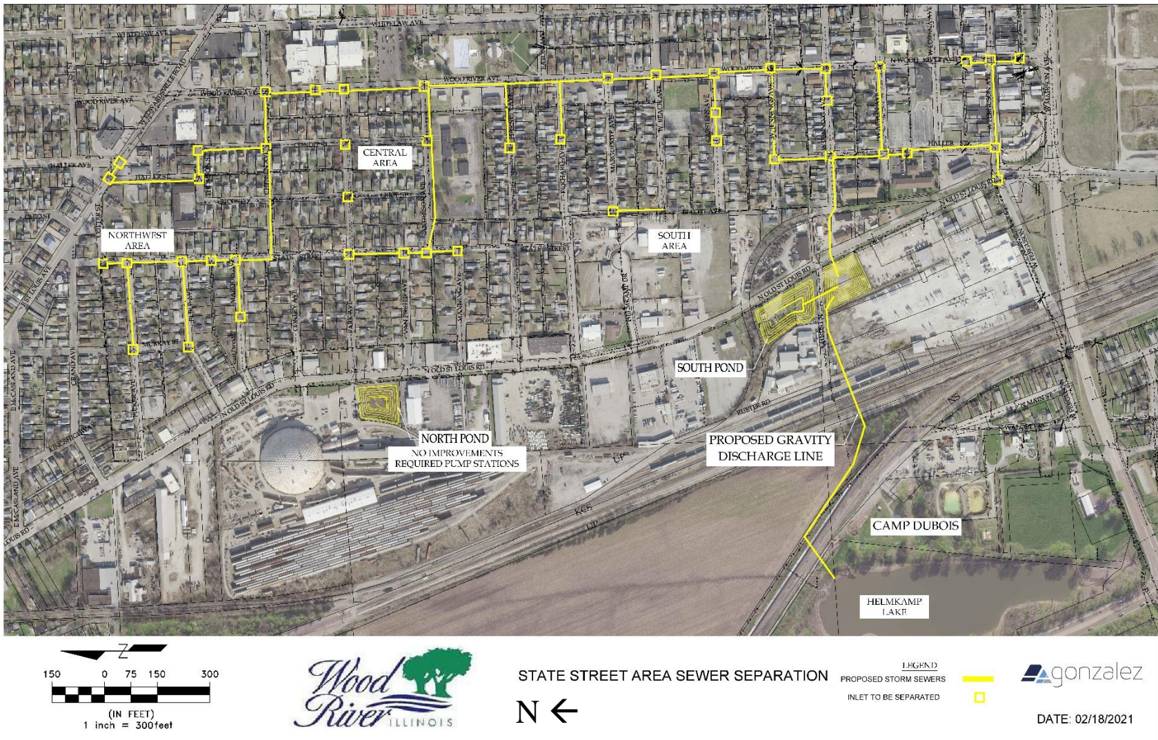
Figure 2. Proposed project features needed to separate the combined sewer and storm water systems.
