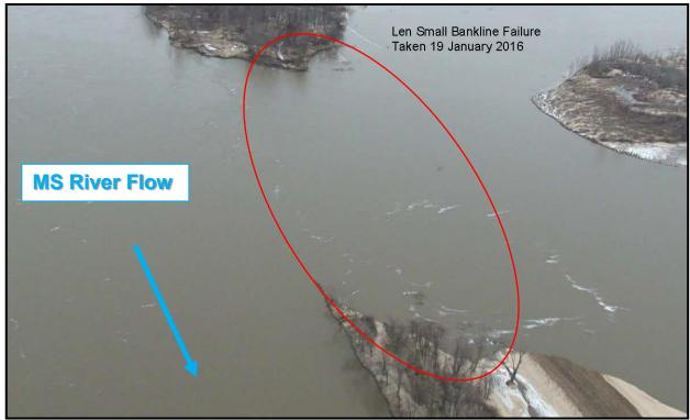
Figure 3. Bankline failure during January 2016
