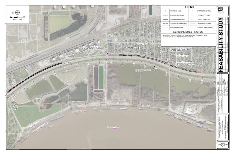
Figure 4. Proposed features for reach 3 for the Standards Plan and Standards Plan with Reach Screening Alternatives.
