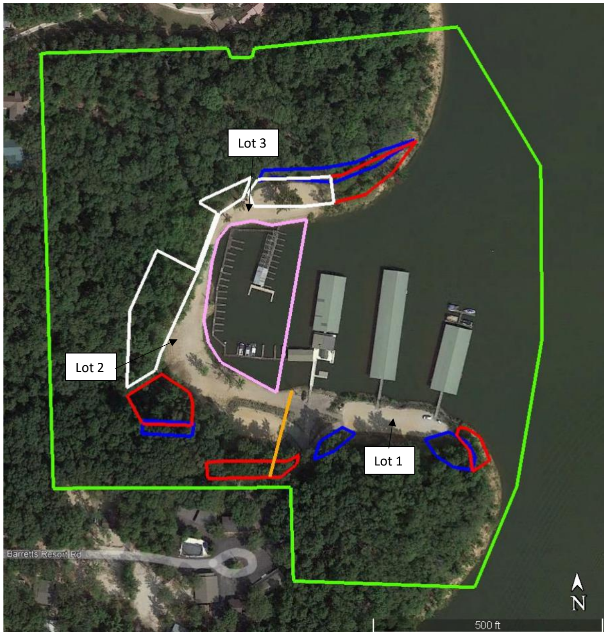
Figure 1. Proposed Action Alternative project area (green), material removal (blue) and placement (red and white), waterline replacement (orange), and lake dredging (pink) for the Wappapello Lakeside Marina Expansion project.
