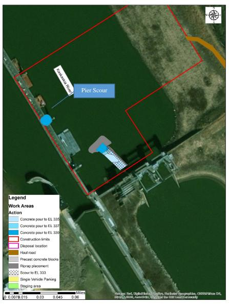
Figure 2. Details of the proposed excavation and fill needed to repair scour hole.
