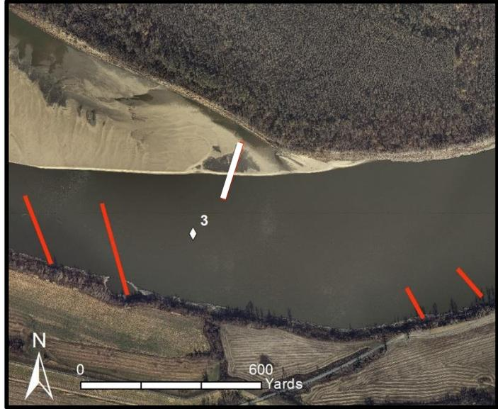
Figure 8. 2012 Aerial imagery of the Eliza Point-Greenfield Bend Phase 3 work area, including the new rootless dike structure (white), and bendway weirs along the right bank (red).
