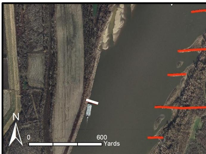
Figure 9. 2012 Aerial imagery of the Dogtooth Bend Phase 5 work area, including the new river training structure (white), and existing river training structures.
