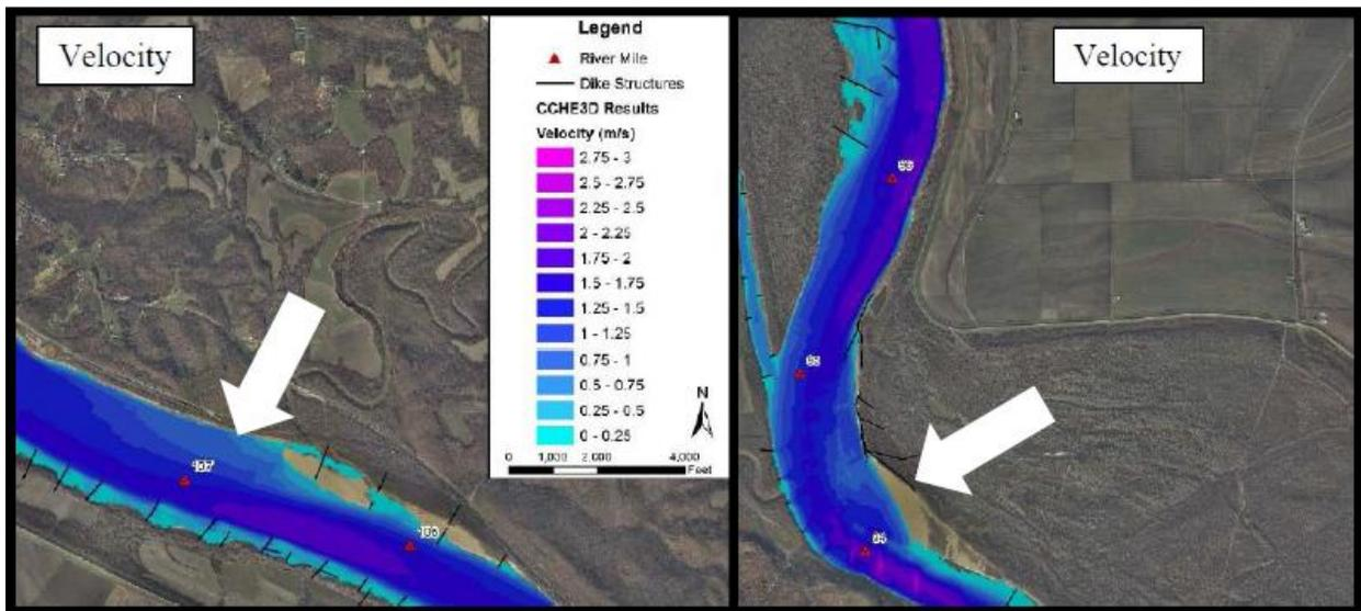
Figure 6. Example of sites from the 3-D model used to supplement pre-construction velocity HSI scores. HSI scores of 0.75 (left) and 0.51 (right) were developed from the unstructured MCB sandbar and point bar habitat indicated by the arrows.
