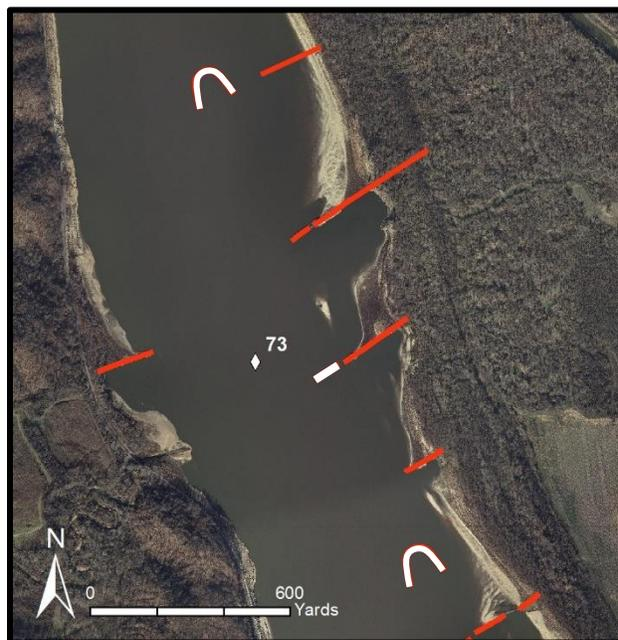
Figure 11. 2012 Aerial imagery of the Grand Tower Phase 5 - Crawford Chevrons work area, including new river training structures (white), and existing river training structures (red).
