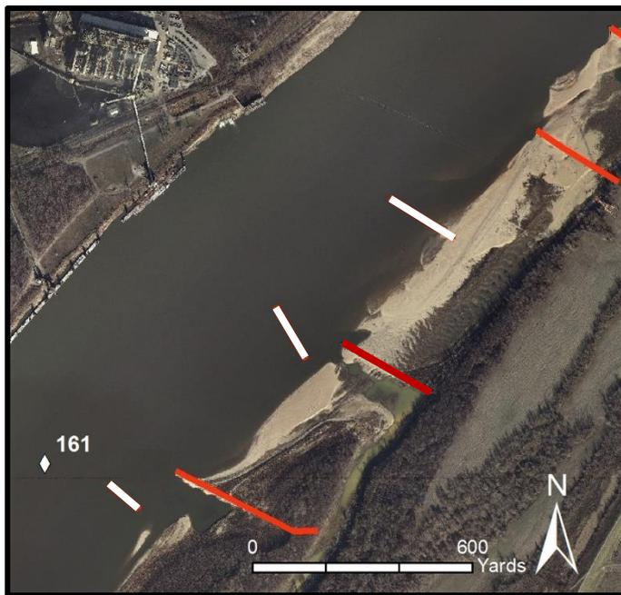
Figure 10. 2012 Aerial imagery of the Mosenthein-Ivory Landing Phase 5 work area, including the new rootless dike structures (white), and existing river training structures.
