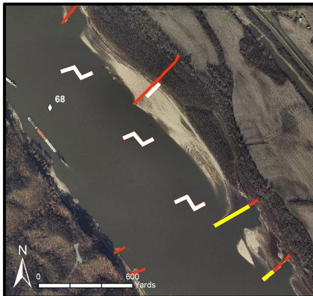
Figure 12. 2012 Aerial imagery of the Grand Tower Phase 5 - Vancill Dikes work area, including new river training structures (white) structure removal (yellow), and existing river training structures.
