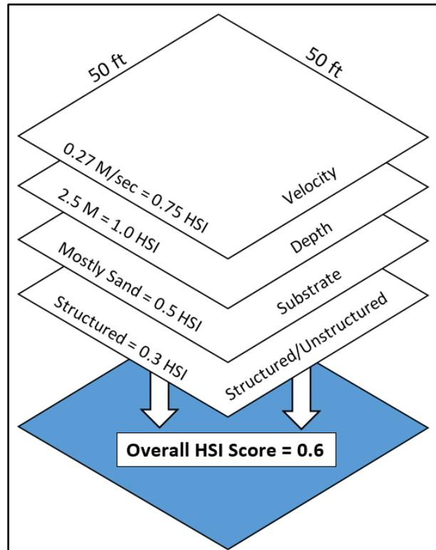
Figure 4. Conceptual model of HSI score calculation process for a 50ft x 50ft cell within a work area. Example data and resulting HSI scores are included for demonstration. Refer to model parameters (Figure 2) for explanation of specific score calculations.
